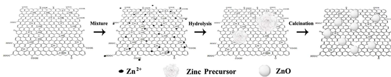
Fig. 1 Schematic presentation of the fabrication of rGO-ZnO.
