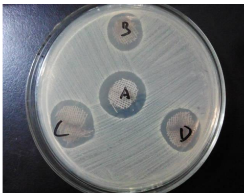
Figure 5. Diagram of inhibition zone experiment against S. aureus ATCC 25923 using cotton fabrics dripped by Ag/SA composites solution (0.57mg/mL nanosilver) after a certain number of washing. A: 0 time, B: 2 times, C: 5 times, D: 10 times.
