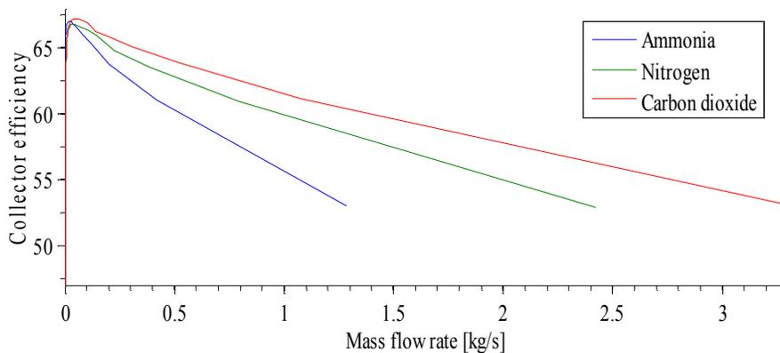
Figure 10. Effect of fluid mass flow rate on the collector efficiency
