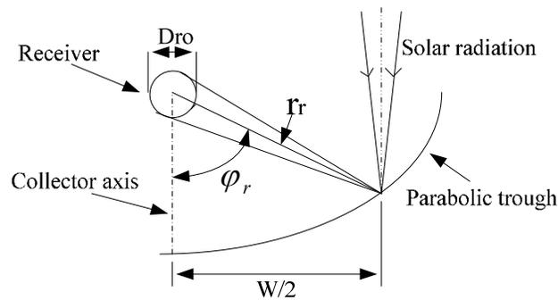
Figure 2 (a). Schematic diagram of a parabolic trough system
