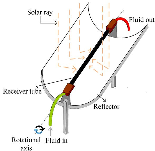
Figure 1. Parabolic trough concentrating solar system
