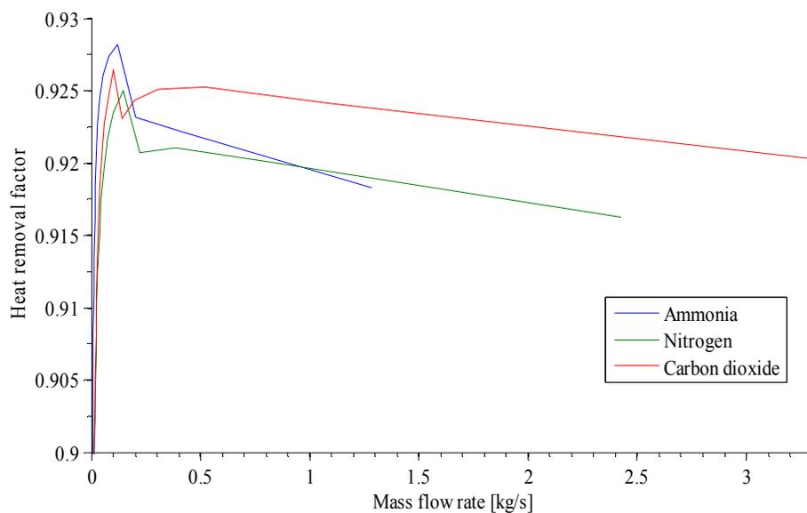
Figure 9. Effect of fluid mass flow rate on heat removal factor
