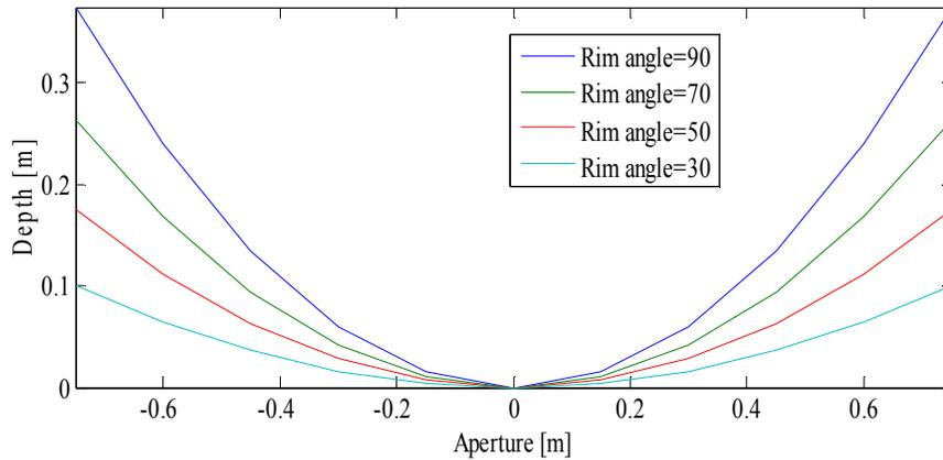
Figure 2(b). Profile of parabolic trough at various rim angles
