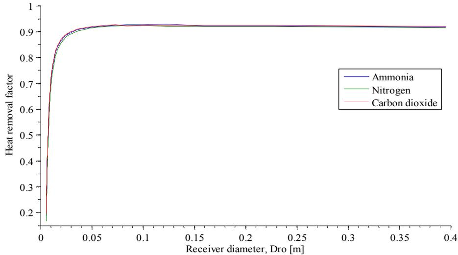
Figure 8. Effect of receiver size on heat removal factor
