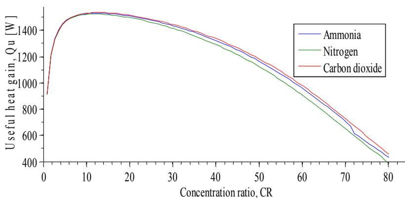
Figure 6(a). Effect of concentration ratio on useful heat gain
