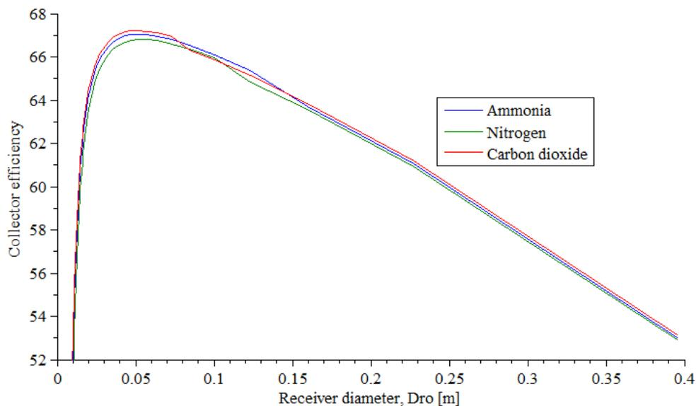
Figure 5(b). Effect of receiver sizes on collector efficiency
