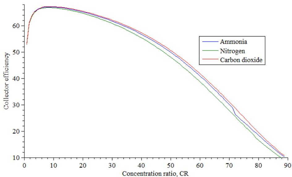
Figure 5(a). Effect of concentration ratio on collector efficiency
