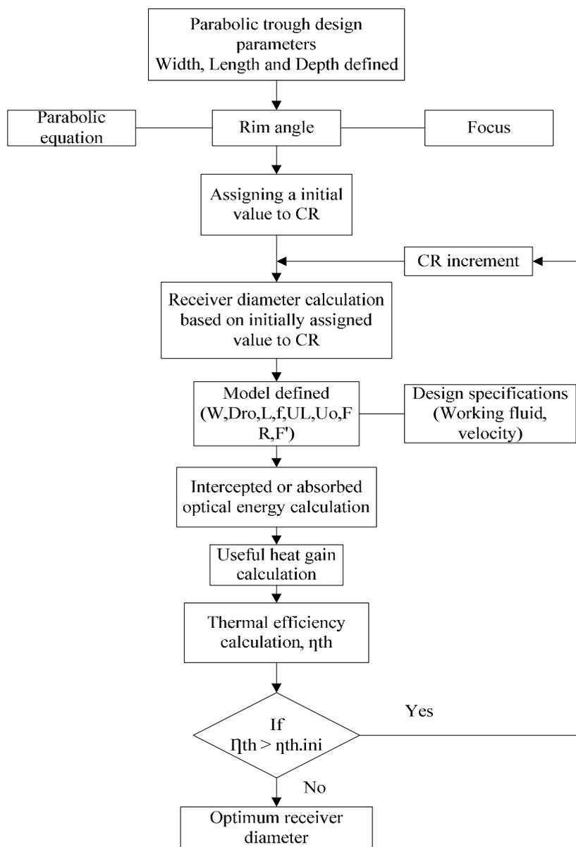
Figure 4. Outline of the procedure for optimizing the receiver size
