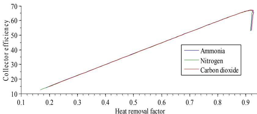
Figure 7. Effect of heat removal factor on collector efficiency
