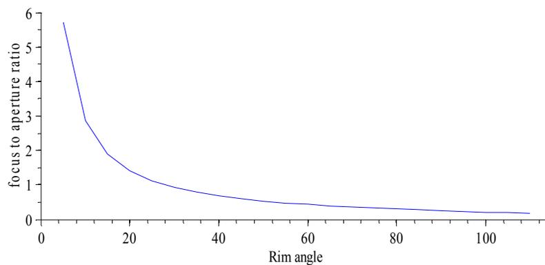
Figure 3. Ratio of focus-to-aperture versus rim angle
