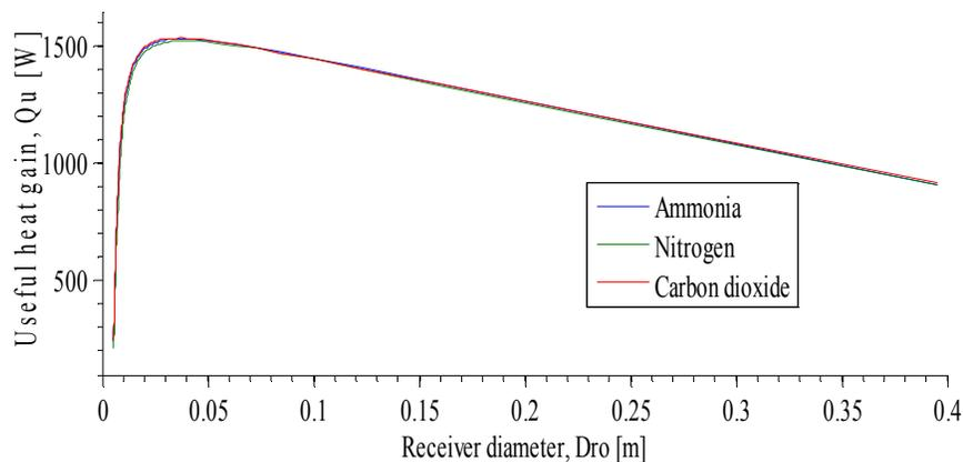
Figure 6(b). Effect of receiver sizes on useful heat gain
