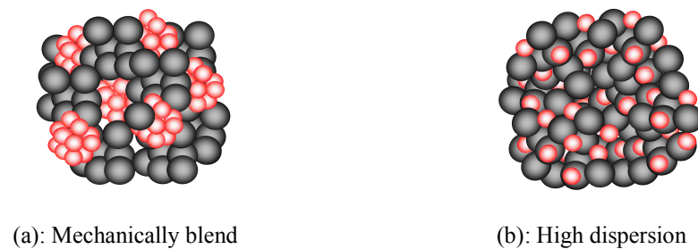
Fig.11. The patterns of catalyst contacting with the coal.
