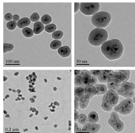
Figure 3 TEM images of  $\text{Fe}_3\text{O}_4@\text{SiO}_2$  (up) and  $\text{Fe}_3\text{O}_4@\text{SiO}_2\text{-NH}_2$  (down).
