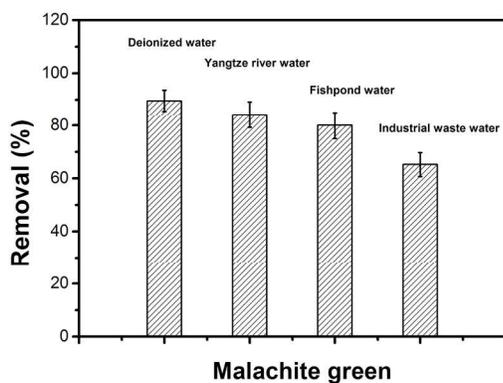
Figure 8 The removal efficiency of malachite green in different water samples. The initial concentration of malachite green and  $\text{Fe}_3\text{O}_4@\text{SiO}_2\text{-NH}_2$  was 10 mg/L and 100 mg/L, respectively.
