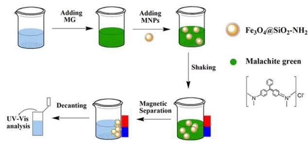
Scheme 1 Schematic illustration of the adsorption process for the malachite green using  $\text{Fe}_3\text{O}_4@\text{SiO}_2\text{-NH}_2$ .
