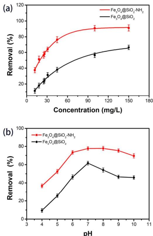
Figure 4(a) The removal of malachite green at different concentrations of  $\text{Fe}_3\text{O}_4@\text{SiO}_2$  and  $\text{Fe}_3\text{O}_4@\text{SiO}_2\text{-NH}_2$ . (b) Effect of pH on the removal efficiency. The concentration of the adsorbent was 100mg/L and the initial concentration of dye solution was 10 mg/L.
