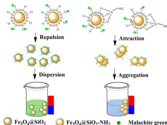
Scheme 2 Schematic illustration of the adsorption process for the malachite green using  $\text{Fe}_3\text{O}_4@\text{SiO}_2\text{-NH}_2$  and  $\text{Fe}_3\text{O}_4@\text{SiO}_2$  at pH 7.
