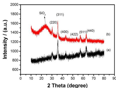
Figure 1 XRD patterns of (a)  $\text{Fe}_3\text{O}_4$ , (b)  $\text{Fe}_3\text{O}_4@\text{SiO}_2$ .
