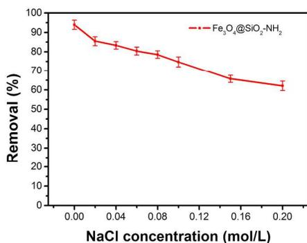
Figure 5 The effect of NaCl concentration on adsorption of malachite green on  $\text{Fe}_3\text{O}_4@\text{SiO}_2\text{-NH}_2$ .
