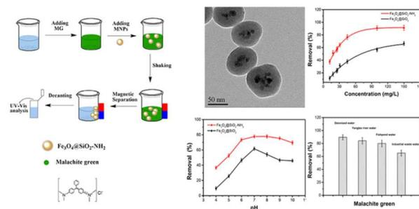
A novel magnetic adsorbent with an amino-modified  $\text{SiO}_2$ -coated  $\text{Fe}_3\text{O}_4$  magnetite was prepared. Under the optimal conditions, the removal efficiency of malachite green is over 90% by the  $\text{Fe}_3\text{O}_4@\text{SiO}_2\text{-NH}_2$ .
