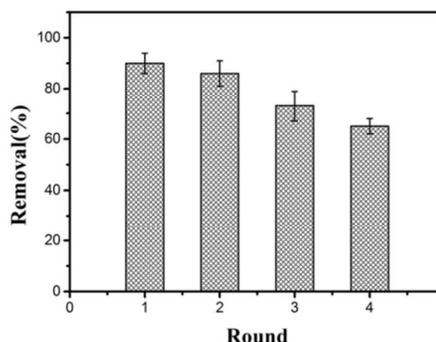
Figure 7 Recycling of Fe<sub>3</sub>O<sub>4</sub>@SiO<sub>2</sub>-NH<sub>2</sub> in the removal of dyes. The initial concentration of malachite green solutions was 10 mg/L and that of Fe<sub>3</sub>O<sub>4</sub>@SiO<sub>2</sub>-NH<sub>2</sub> was 100 mg/L.
