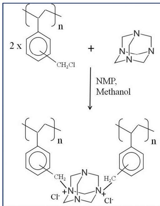
**Scheme 1** Synthesis scheme of cross-linked anion exchange polymer.
