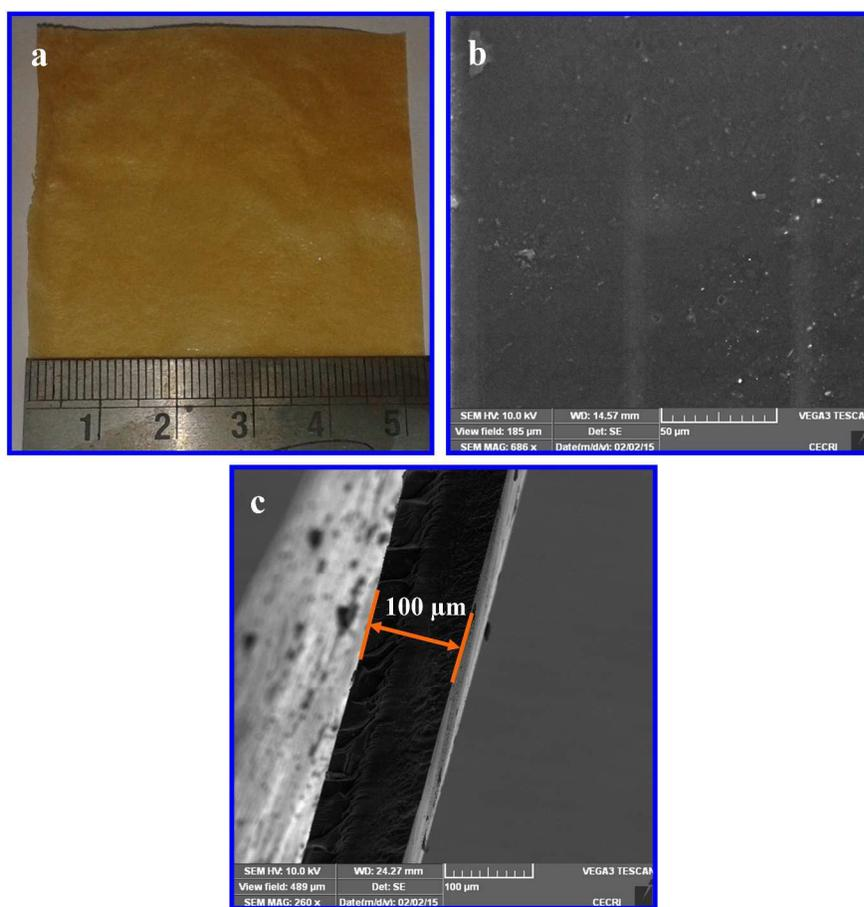
**Fig. 5** (a) Optical image; (b) Surface and (c) cross-sectional SEM images of the quaternized PVBC membrane (HMTA / PVBC = 0.33 : 1).
