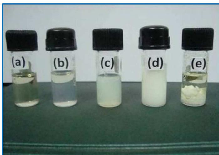
**Fig. 3** Photograph of the quaternized anion exchange polymers with different HMTA / PVBC ratios (a) 0 : 1; (b) 0.2 : 1; (c) 0.33 : 1; (d) 0.5 : 1; (e) 1 : 1 in THF.
