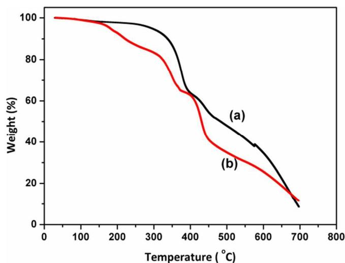
**Fig. 4** Thermo-gravimetric curves of (a) PVBC and (b) Quaternized PVBC in Cl<sup>-</sup> form (HMTA / PVBC = 0.25 : 1).
