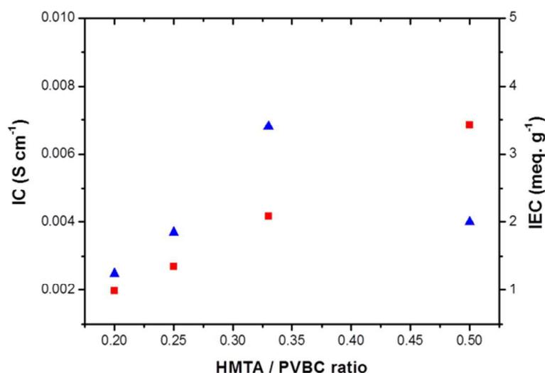
**Fig. 6** Ionic conductivity ( $\blacktriangle$ ) and Ion-exchange capacity ( $\blacksquare$ ) of anion exchange membranes with different HMTA / PVBC ratios at 25 °C.
