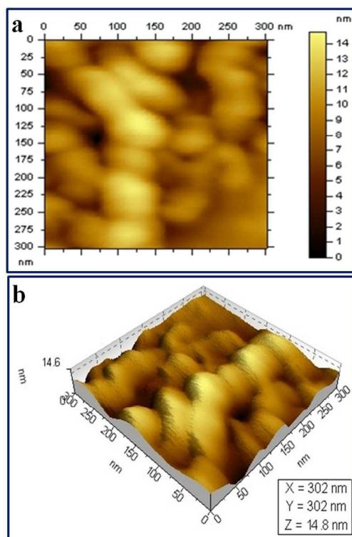
**Fig. 7** AFM tapping mode: (a) topography image and (b) 3D phase image of anion exchange membrane (HMTA / PVBC = 0.33 : 1).
