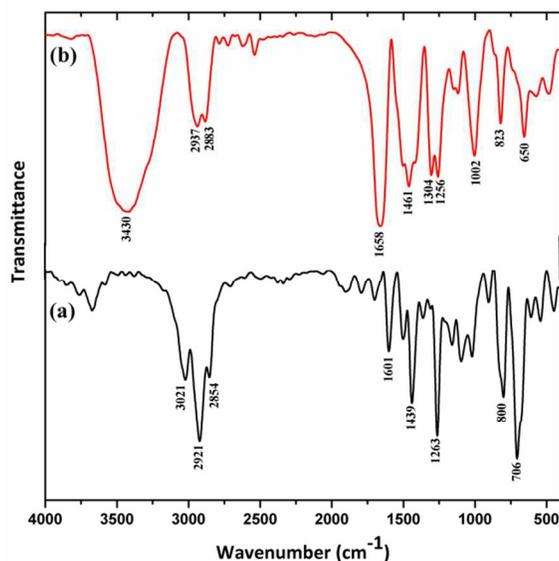
**Fig. 1** FT-IR Spectra of (a) PVBC and (b) Quaternized PVBC in  $\text{OH}^-$  form (HMTA / PVBC = 0.5 : 1).
