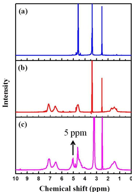
**Fig. 2**  $^1\text{H-NMR}$  Spectra of (a) HMTA; (b) PVBC and (c) Quaternized PVBC in Cl<sup>-</sup> form (HMTA / PVBC = 0.5 : 1)
