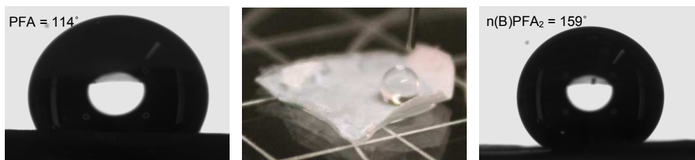
Figure 11. Hydrophobicity enhancement of the fluorinated surface (PFA) after nanostructuring by AAO templates.
