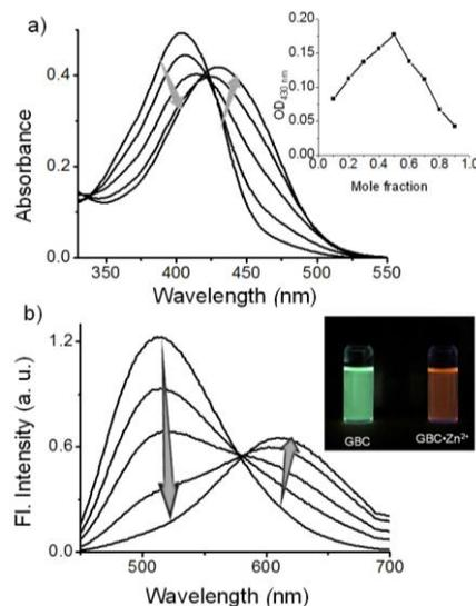
Fig. 2 Changes in the a) absorption and b) emission spectra of GBC (6  $\mu$ M) with the addition of Zn(ClO<sub>4</sub>)<sub>2</sub> (0-6  $\mu$ M) in 1:1 acetonitrile/water (HEPES, pH 7.2,  $\lambda_{exc.}$  at 422 nm). Inset in Fig. a) shows the Job's plot showing 1:1 binding of GBC to Zn(ClO<sub>4</sub>)<sub>2</sub> in acetonitrile/water (1:1 v/v, HEPES buffer, pH 7.2). Inset in Fig. b) shows the fluorescence colour change of GBC in the absence and presence of Zn<sup>2+</sup>.
