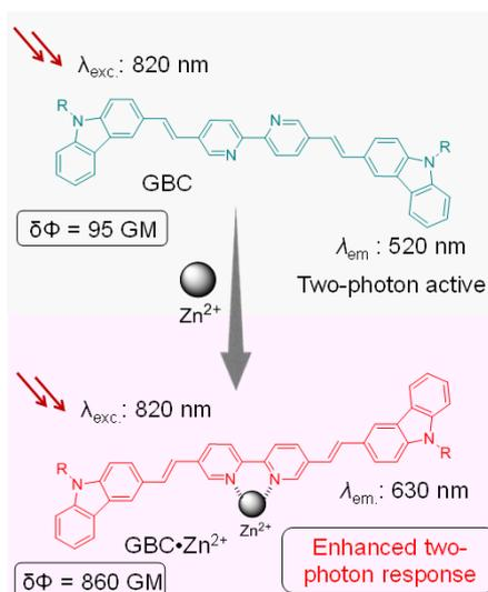
Fig. 1 Schematic representation of two-photon response of GBC and GBC·Zn<sup>2+</sup>
