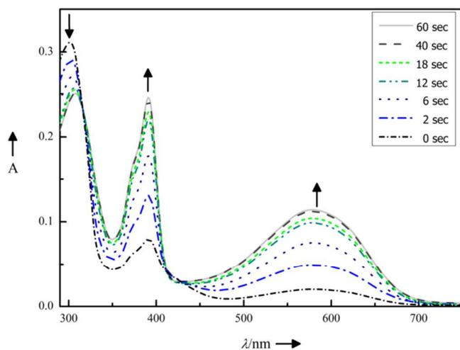
**Figure 3.** Photochromic properties of compound **11** (10  $\mu$ m in DMSO): Absorption spectra changes upon continuous irradiation for 0, 2, 6, 12, 18, 40 and 60 s with light of  $\lambda_{\max} = 312$  nm.
