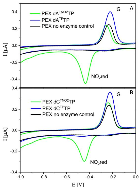
**Figure 7.** Detail of CV responses at HMDE of PEX products synthesized with temp<sup>md16</sup> template and dNTP mixes containing dN<sup>Tx</sup>TP conjugate (as specified in legend) complemented with three respective unmodified 5 dNTPs. For full CV scans and other details see Figure S16-S17 and Experimental section.
