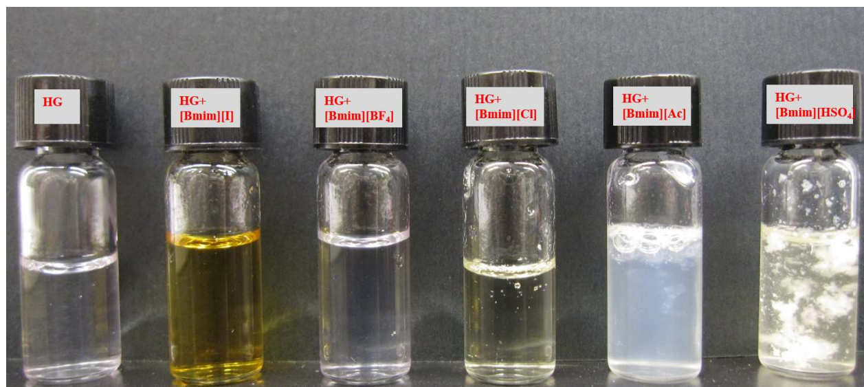
Fig. 3 Optical image for 1 wt% PNIPAM-co-AA hydrogel in water in the presence of different kinds of ILs at the concentration of 1.5 M.
