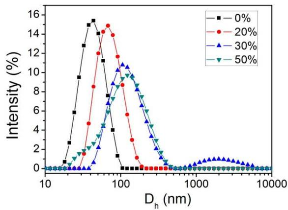
**Fig. 3** Hydrodynamic diameters ( $D_h$ ) of  $M_{93}A_{94}$  in solution ( $0.2 \text{ mg mL}^{-1}$ ) with different DMF-water mixture solvents ( $x \%$ , volume content of water).
