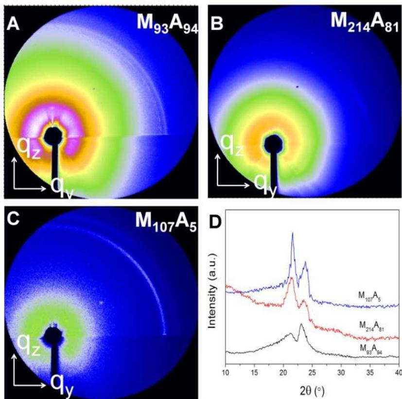
**Fig. 7** Two-dimensional GIXRD patterns (2D GIXRD: A-C) and the out-of-plane XRD profiles of PM-*b*-PAA films spin-coated from 2 mg mL<sup>-1</sup> DMF solution (D).
