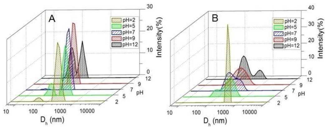
**Fig. 4** Hydrodynamic diameters ( $D_h$ ) of  $M_{214}A_{81}$  (A) and  $M_{107}A_5$  (B) in water ( $0.2 \text{ mg mL}^{-1}$ ) with different pH value of 2, 5, 7, 9, 12, respectively.
