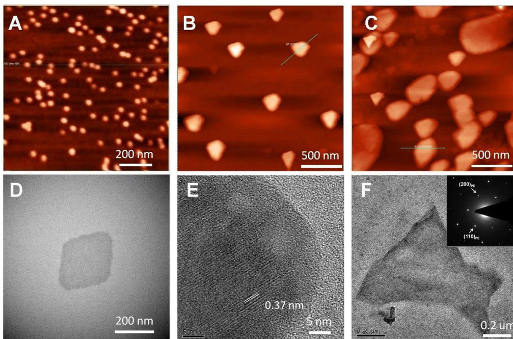
**Fig. 8** AFM height images of  $M_{93}A_{94}$  during the controlled growth in  $0.2 \text{ mg mL}^{-1}$  dilute DMF solution for 0 h (A), 12 h (B), 24 h (C) at  $50 \text{ }^\circ\text{C}$ ; TEM micrographs of  $M_{93}A_{94}$  (D, E) and  $M_{214}A_{81}$  (F) crystals during the controlled growth from  $0.2 \text{ mg mL}^{-1}$  DMF solution for 24 h; the inset in (F) is the corresponding SAED pattern.
