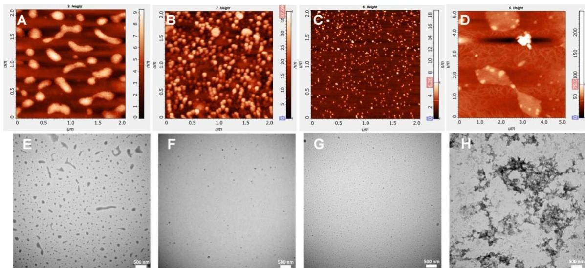
**Fig. 5** AFM height images (A-D) and TEM images (E-H) of  $M_{93}A_{94}$  micelles prepared from  $0.2 \text{ mg mL}^{-1}$  solution with different pH values: (A, E) pH = 2, (B, F) pH = 5, (C, G) pH = 7, (D, H) pH = 12.
