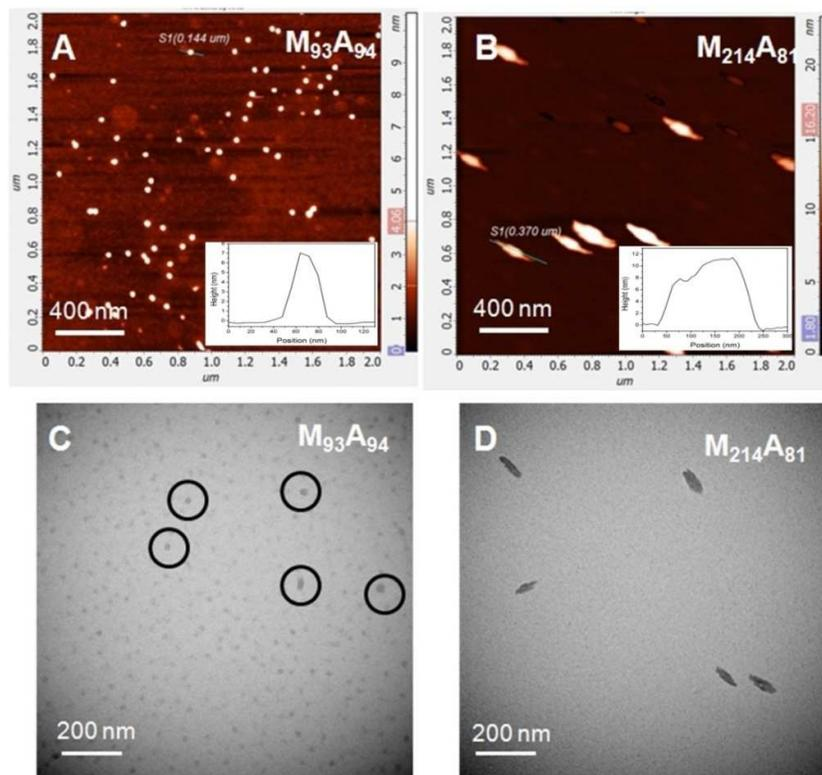
**Fig. 1** AFM height images (A, B) and TEM micrographs (C, D) of PM-*b*-PAA micelles prepared from 0.2 mg mL<sup>-1</sup> DMF solution. The insets are cross-section profiles of the marked positions corresponding to the height images.
