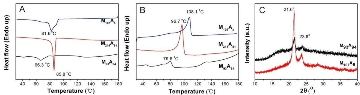
**Fig. 6** DSC cooling (A) and re-heating (B) traces of PM-*b*-PAA powder; XRD patterns (C) of freeze-dried  $M_{93}A_{94}$  and  $M_{107}A_5$  samples.
