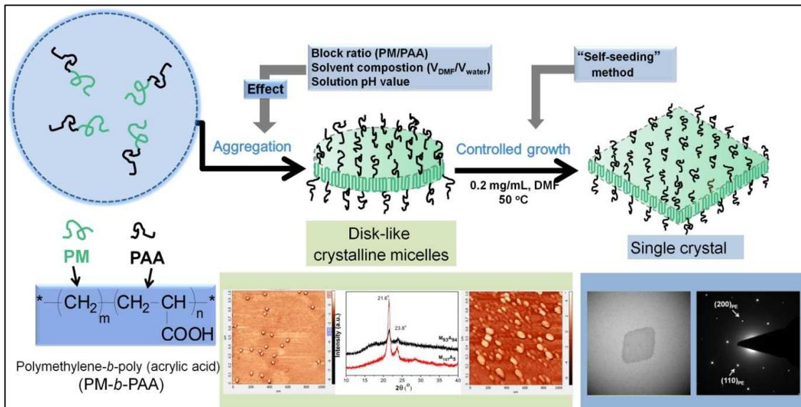
**Fig. 9** Schematic representation of the aggregation behavior and the controlled growth of PM-*b*-PAA micelles with confined crystallization.
