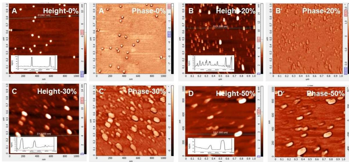
**Fig. 2** AFM height (A-D) and phase images (A'-D') (scan size:  $1 \mu\text{m} \times 1 \mu\text{m}$ ) of  $M_{93}A_{94}$  micelles prepared from  $0.2 \text{ mg mL}^{-1}$  solution with different DMF-water mixture solvents (x %, volume content of water). The insets are cross-section profiles of the marked positions in the corresponding height images.
