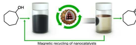
Scheme 2. Magnetic separation and recycling of the designed Pd nanocatalysts.
