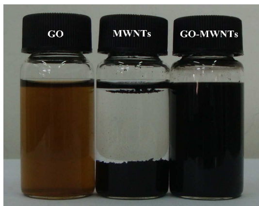
Fig. 2 Digital camera images of the aqueous dispersibility of GO, MWNTs and GO-MWNTs.
