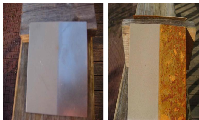
Fig. 9 Photographs depicting coated (left) and non-coated (right) steel plates taken after exposure to atmosphere for about 60 days (adapted from www.ornl.gov/File%20Library/.../06-Superhydrophobic_Materials.pdf ).
