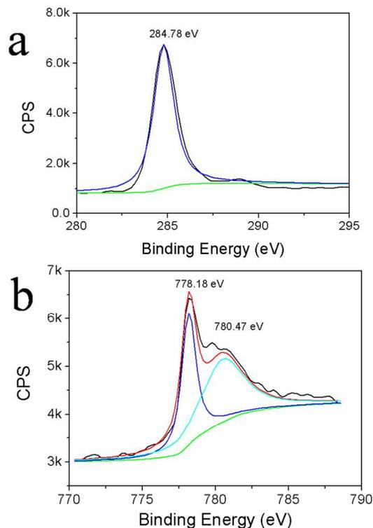
**Fig.3** (a) C 1s (b) Co 2p XPS traces of the Co@C NPs.
