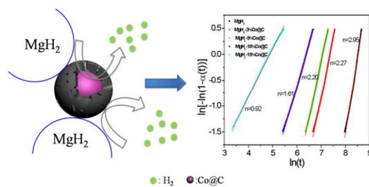
Core-shell Co@C shows excellent catalytic effects on MgH<sub>2</sub>. JMA modeling find that desorption of MgH<sub>2</sub> gradually happens along lower-dimension with increase of Co@C.
