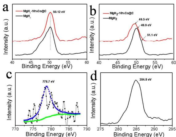
**Fig.9** XPS spectra of (a) as-milled and (b) after dehydrogenated Mg 2p peaks. (c) Co 2p and (d) C 1s patterns of the dehydrogenated MgH<sub>2</sub>-10%Co@C sample.
