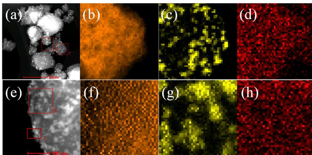
**Fig. 4** Representative STEM images of the  $\text{MgH}_2$ -10%Co@C samples (a-d) as-milled, (e-f) after dehydrogenated. Mg, Co and C elements mapping are in brown, yellow and red, respectively.
