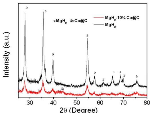
**Fig.7** XRD images of the as-milled pure MgH<sub>2</sub> and MgH<sub>2</sub>-10%Co@C samples.
