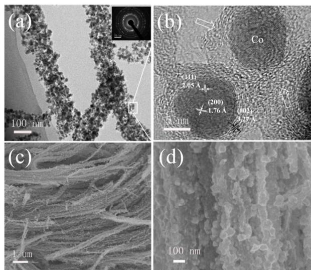
**Fig.1** (a) TEM, (b) HRTEM and (c-d) SEM images in different resolution of the as-prepared Co@C sample. Insert (a) is the SAED pattern.
