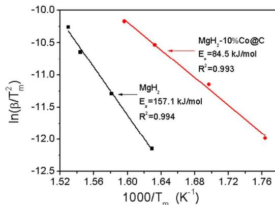
**Fig.8**  $E_a$  of the as-prepared pure MgH<sub>2</sub> and MgH<sub>2</sub>-10%Co@C composites, obtained by Kissinger method at the heating rate of 2, 5, 10, 15 °C min<sup>-1</sup>.
