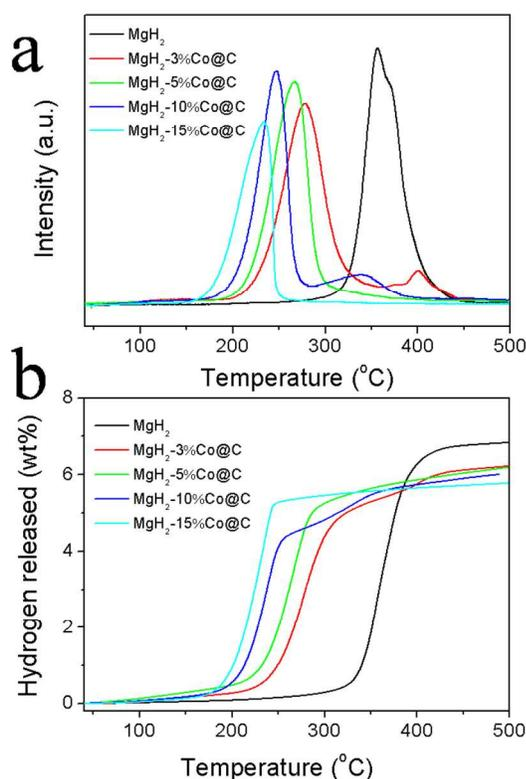
**Fig.5** (a) Thermal desorption curves and (b) the corresponding hydrogen desorption patterns of as-prepared pure  $\text{MgH}_2$  and 3 wt%, 5 wt%, 10 wt%, 15 wt%  $\text{Co@C}$  doped  $\text{MgH}_2$  samples. Heating at  $2^\circ\text{C min}^{-1}$  under Ar atmosphere
