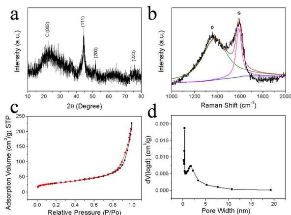
**Fig.2** (a) XRD, (b) Raman, (c) nitrogen sorption isotherms and (d) the corresponding pore width distribution pattern of Co@C sample.
