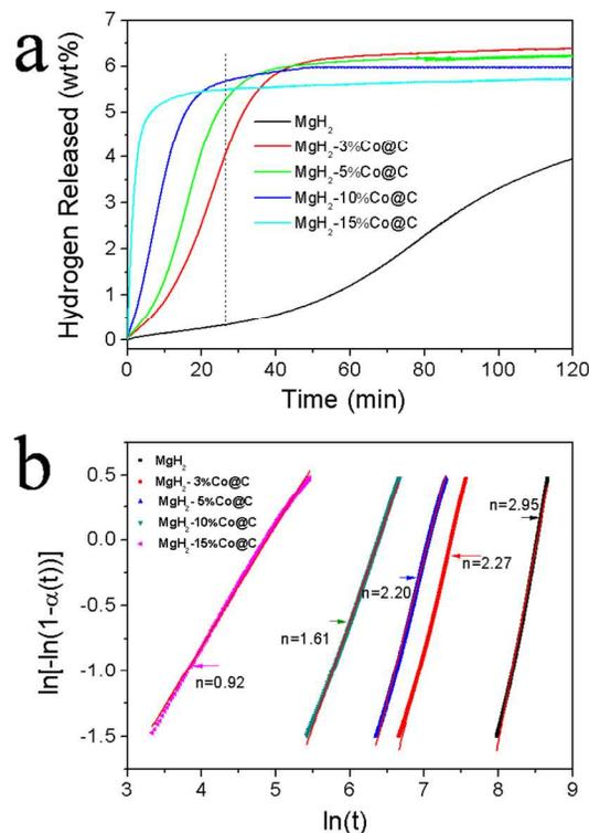
**Fig.6** (a) Isothermal dehydrogenation curves of the pure  $\text{MgH}_2$ ,  $\text{MgH}_2$ -3% $\text{Co@C}$ ,  $\text{MgH}_2$ -5% $\text{Co@C}$ ,  $\text{MgH}_2$ -10% $\text{Co@C}$  and  $\text{MgH}_2$ -15% $\text{Co@C}$  composites at  $300^\circ\text{C}$  and (b) their JMA fitting plots.
