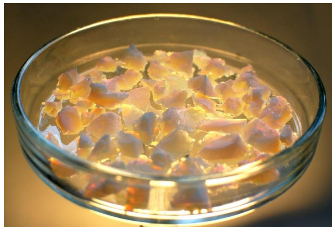
Fig. 5. Photograph of as-synthesized closely packed FeZSM-5 nanozeolite pellets on a Petri dish.
