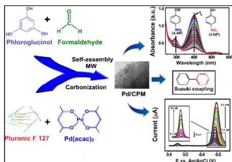
Scheme 1 Schematic illustrations of synthesis and applications of Pd/CPM catalyst system.
