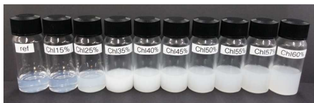
Fig. 2 Silica nanoparticle ( \sim 10 nm) dispersion with increasing chloroform content. The reference sample ("ref") was prepared by mixing silica nanoparticle solution and acidic silica sol (9:1 based on solid weight), and the samples were prepared by adding chloroform to this reference solution in quantities between 15 and 60 wt%.
