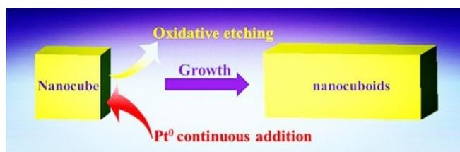
**Fig. 4** The schematic illustration of the mechanisms responsible for the formation of Pt nanocuboids.
