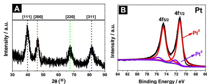
**Fig. 2** (A) XRD pattern of Pt nanocuboids. (B) XPS spectrum of Pt nanocuboids in the Pt 4f region.
