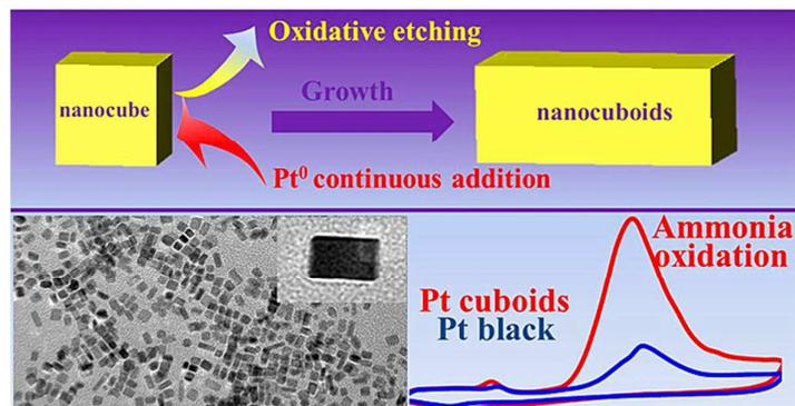
Pt-nanocuboids were synthesized by the simple hydrothermal method with the assistance of L-Lysine, exhibiting enhanced catalytic activity towards ammonia oxidation.
