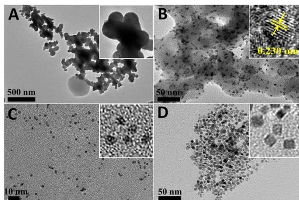
**Fig. 3** TEM images of the product prepared using the standard procedure except for the exclusion of (A) PVP, (B) HCHO and (C) L-Lysine. (D) TEM image of Pt nanocrystals prepared by displacing the air with N<sub>2</sub> to eliminate typical etchant O<sub>2</sub>. The top-right insets in Figure 3A-D show the corresponding magnified Pt nanoparticles.
