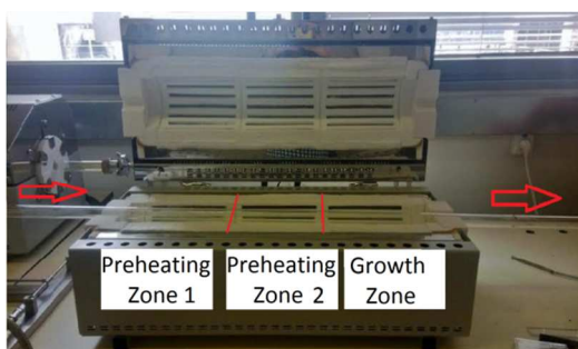
Fig. 1 Sketch of the three-zone furnace. Every zone is heated independently. The gases flow from left to right: in the first two zones the gas mixture is preheated, in the third zone lays the sample where graphene growth takes place.
