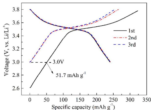
Fig. 2 The charge and discharge profiles in the initial three cycles. The capacity is calculated based on the weight of LiBr in the cathode
