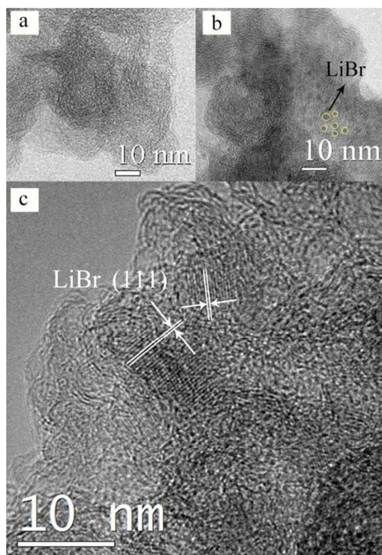
Fig. 1 HRTEM image of the CCB substrate (a); HRTEM images of the as-prepared LiBr-CCB composite (b and c).
