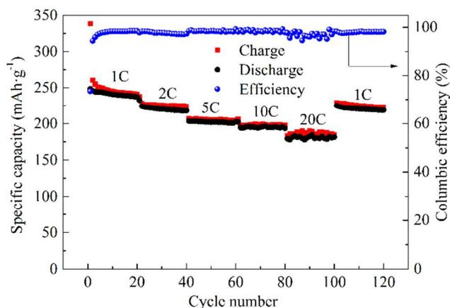
Fig. 4 The cycle performance of LiBr-CCB/lithium cell at various charge-discharge rates. The capacity is calculated based on the weight of LiBr in the composite
