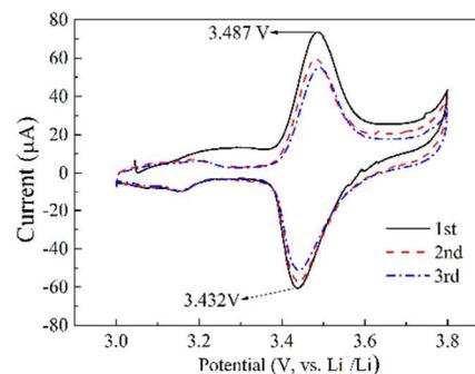
Fig. 3 Cyclic voltammograms of the LiBr-CCB composite at the scan rate of 0.1 mV s<sup>-1</sup> in the initial 3 cycles.
