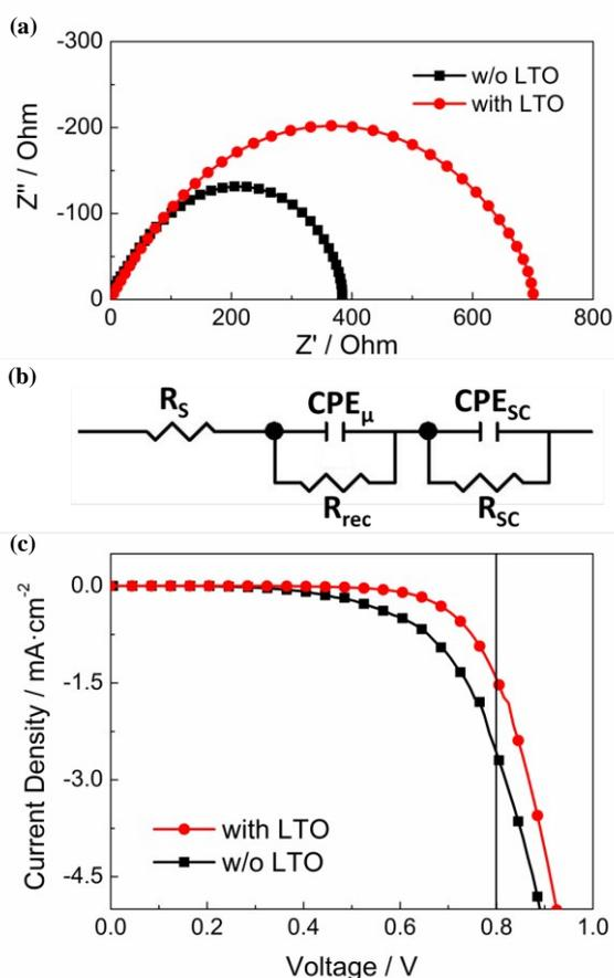
Figure 8. (a) Nyquist plots of EIS measurements under dark condition with a 0.8 V bias voltage (b) Equivalent circuit model used for EIS analysis ( $R_s$  and  $R_{rec}$  are the series resistance and recombination resistance of device,  $CPE_{\mu}$  is the chemical capacitance of films and  $R-CPE_{sc}$  is the impedance of selective contacts), (c) Dark current curve of devices with (red) and without (red) LTO modification.
