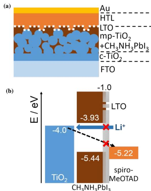
Figure 4 Schematic of (a) device architecture and (b) the relative energy levels of each layer of the perovskite solar cells
