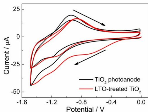
Figure 6. First two scans of CVs with TiO<sub>2</sub> (black) or LTO-treated TiO<sub>2</sub> (red) working electrodes, Pt counter electrode and Ag reference electrode in 0.1M LiClO<sub>4</sub>/acetonitrile at a scan speed of 50 mV/s. Arrows show the scan directions.
