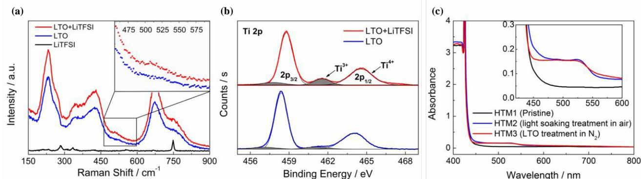
Figure 2. (a) Raman spectrum and (b) Ti 2p XPS of LTO after reaction with LiTFSI in HTM solution, (c) Absorption spectra of HTM1 (pristine HTM solution in N<sub>2</sub>), HTM2 (HTM solution after 10 min light soaking treatment in air) and HTM3 (centrifuged HTM solution after reaction with LTO powder in N<sub>2</sub>). Insets in (a) and (c) show magnified images of the Li-O stretching vibration regions and the oxidized spiro-MeOTAD peak at 520 nm.
