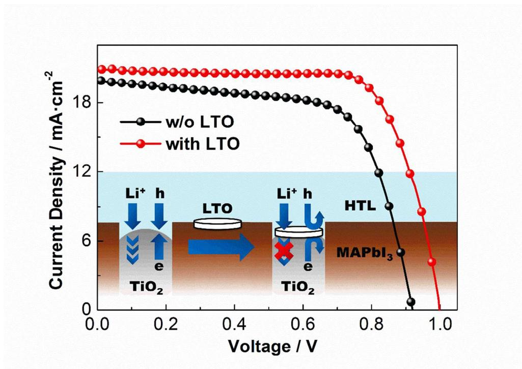
Spinel lithium titanate (LTO) was used as modification material at the perovskite-sensitized TiO<sub>2</sub>/HTL interface, acting as a Li<sup>+</sup> separator to prevent Li<sup>+</sup> intercalation into TiO<sub>2</sub> and reducing carrier recombination.
