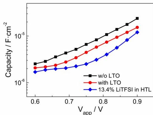
Figure 7. Chemical capacitance extracted at an intermediate frequency of 1000 Hz from EIS of: pristine device (black), with LTO modification (red) and with low LiTFSI molar ratio of 13.4% in the HTL (blue), performed under one sun illumination condition with a 0.8 V bias voltage.
