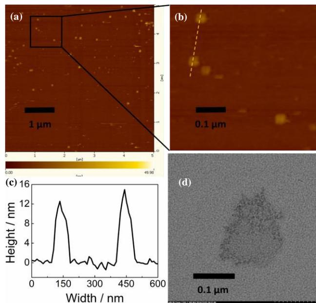
Figure 3 (a) AFM image of deposited LTO nanosheets on silicon substrate, (b) the corresponding magnified image with height information on the orange dash line depicted in (c), (d) TEM image of LTO nanosheets.
