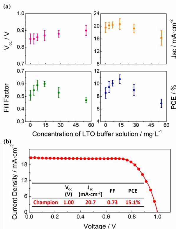
Figure 5. (a) Photovoltaic characteristics for PSCs with LTO modification of different concentration (statistics of data for 10 batches of devices). (b) J-V curve of the champion device with LTO modification. Insert table shows the corresponding photovoltaic characteristics. There are differences of compact  $\text{TiO}_2$  layer preparation methods between (a) and (b) as stated in the experiment part.
