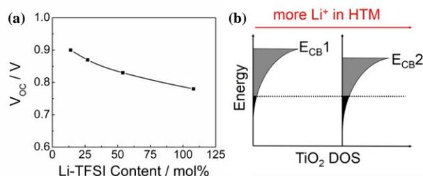
Figure 1. (a)  $V_{\text{OC}}$  characteristics with different Li-TFSI contents in HTL. (b) Schematic of the change of DOS of  $\text{TiO}_2$  with more  $\text{Li}^+$  in HTL.
