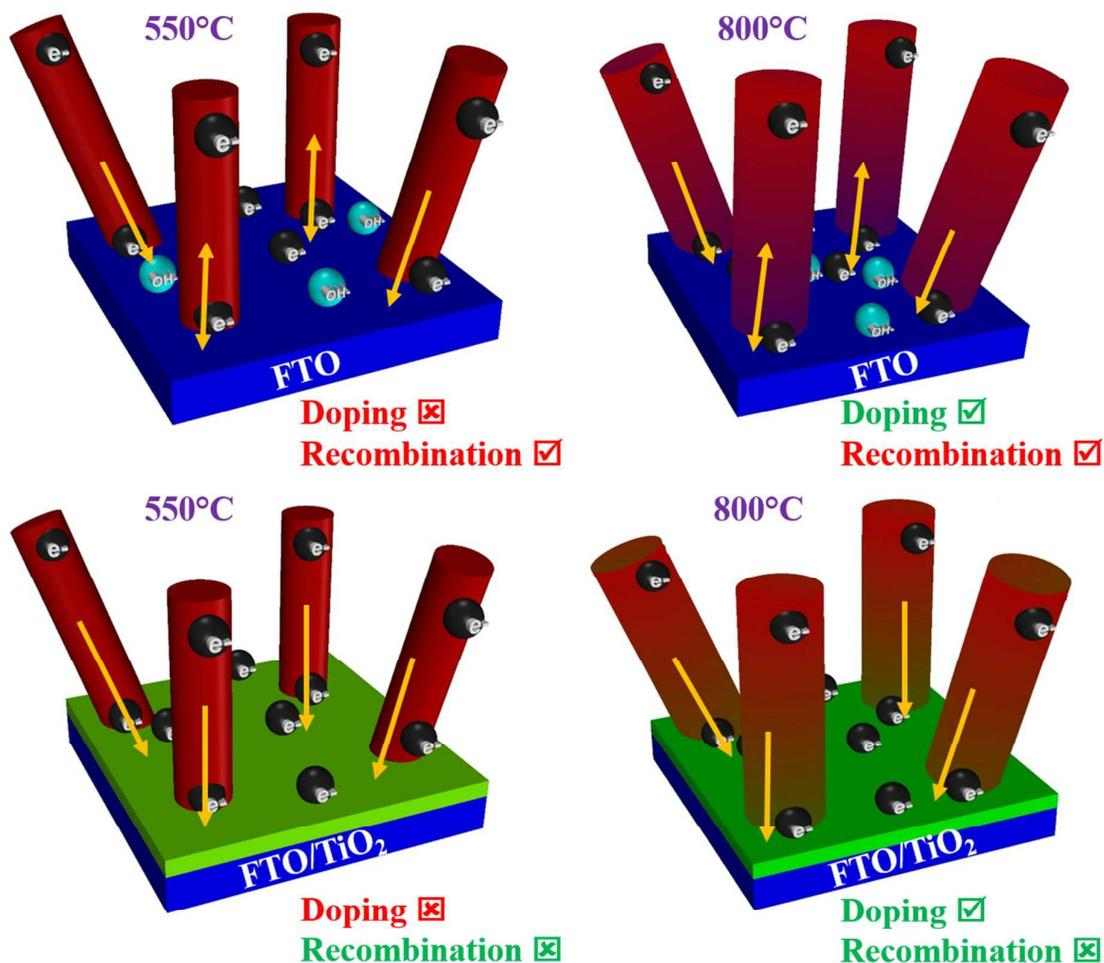
The TiO<sub>2</sub> underlayer effectively suppresses charge recombination at the FTO/ $\alpha$ -Fe<sub>2</sub>O<sub>3</sub> interface and allows Ti<sup>4+</sup> doping apart from Sn diffusion from FTO substrates when sintered at high temperatures (800°C), thus enhancing the charge transport and collection while only charge recombination is suppressed at lower sintering temperatures (550°C).
