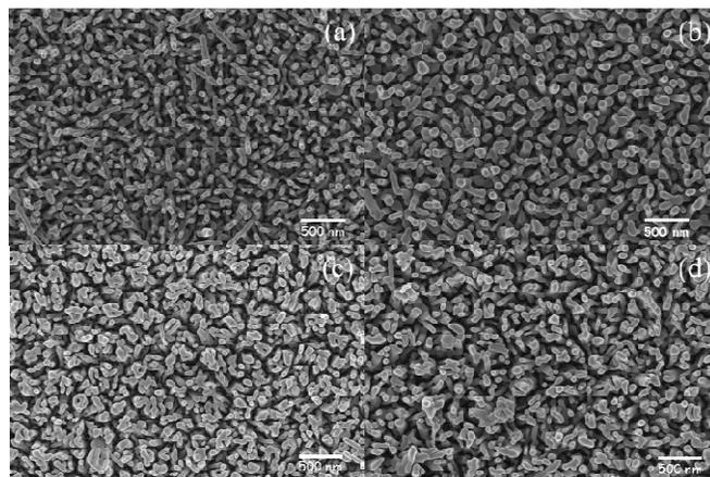
**Fig. 1.** Surface morphology of photoanodes: FTO/α-Fe<sub>2</sub>O<sub>3</sub> nanorods sintered at (a) 550°C, (b) 800°C, and FTO/TiO<sub>2</sub>/α-Fe<sub>2</sub>O<sub>3</sub> nanorods sintered at (c) 550°C and (d) 800°C.
