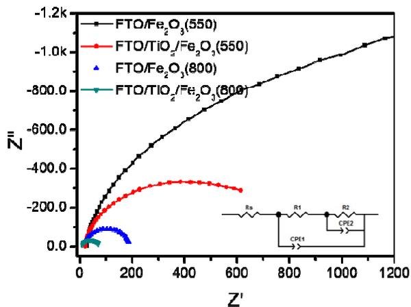
**Fig. 7.** Nyquist plots of FTO/α-Fe<sub>2</sub>O<sub>3</sub> and FTO/TiO<sub>2</sub>/α-Fe<sub>2</sub>O<sub>3</sub> photoanodes sintered at 550 and 800°C using 1 M NaOH under 1-sun illumination conditions. The inset of the Nyquist plot represents the equivalent circuit for EIS.
