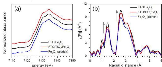
**Fig. 2.** (a) Fe K-edge XANES spectra and (b) Fourier-transforms of Fe K-edge EXAFS for  $\text{FTO}/\alpha\text{-Fe}_2\text{O}_3$  and  $\text{FTO}/\text{TiO}_2/\alpha\text{-Fe}_2\text{O}_3$  photoanodes and reference  $\text{Fe}_2\text{O}_3$  powder.
