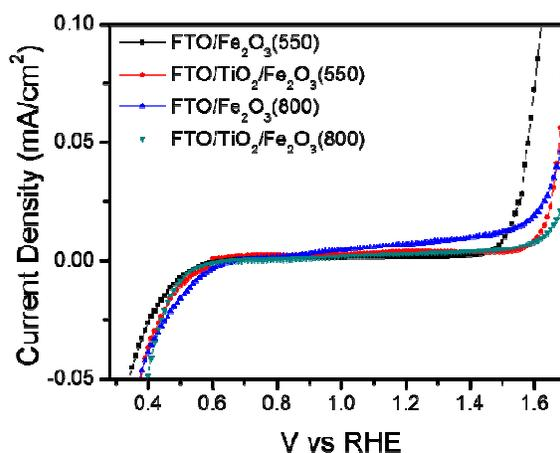
**Fig. 6.** Photocurrent-potential ( $J$ - $V$ ) curves for PEC water oxidation reaction of FTO/ $\alpha$ -Fe<sub>2</sub>O<sub>3</sub> and FTO/TiO<sub>2</sub>/ $\alpha$ -Fe<sub>2</sub>O<sub>3</sub> photoanodes annealed at 550 and 800°C under dark conditions.
