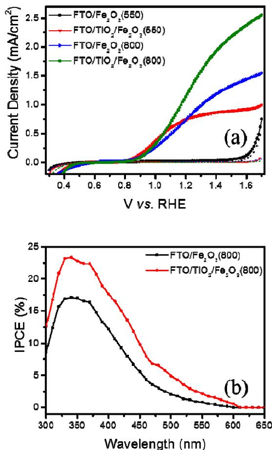
**Fig. 5.** (a) Photocurrent density-potential ( $J$ - $V$ ) curves for PEC water oxidation reaction sintered at 550 and 800°C and (b) IPCE spectra of FTO/ $\alpha$ -Fe<sub>2</sub>O<sub>3</sub> and FTO/TiO<sub>2</sub>/ $\alpha$ -Fe<sub>2</sub>O<sub>3</sub> photoanodes sintered at 800°C using 1 M NaOH under 1 sun standard illumination conditions.
