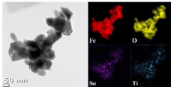
**Fig. 4.** Typical low-magnification TEM image of  $\text{FTO}/\text{TiO}_2/\alpha\text{-Fe}_2\text{O}_3$  photoanodes annealed at 800°C, and its respective elemental mapping images from EELS analysis.
