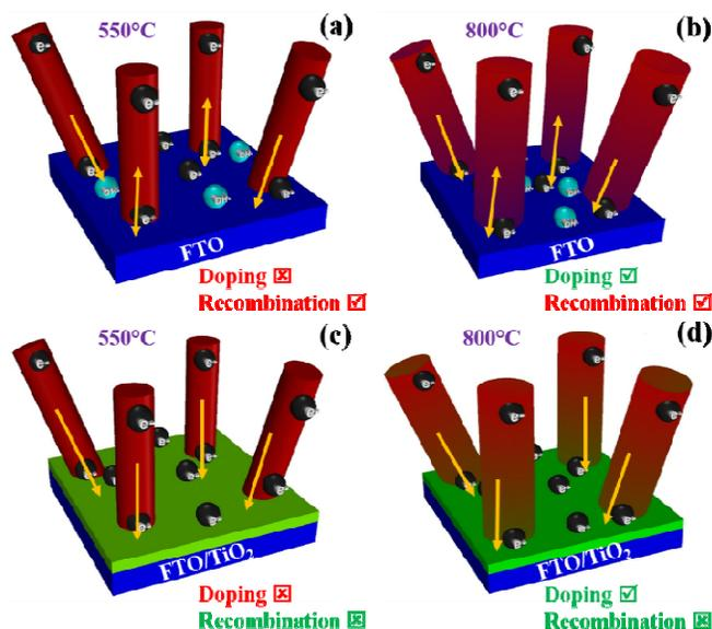
**Scheme 1.** Schematic representation of TiO<sub>2</sub> underlayer effect on hematite photoanodes. (a) and (b) FTO/α-Fe<sub>2</sub>O<sub>3</sub> sintered at 550 and 800°C, (c) and (d) FTO/TiO<sub>2</sub>/α-Fe<sub>2</sub>O<sub>3</sub> sintered at 550 and 800°C, respectively.
