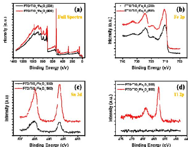
**Fig. 3.** X-ray photoelectron spectra of (a) full scan, (b) Fe 2p, (c) Sn 3d, and (d) Ti 2p recorded from 550°C and 800°C sintered  $\text{FTO}/\text{TiO}_2/\alpha\text{-Fe}_2\text{O}_3$  photoanodes.
