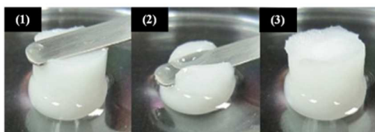
Fig. 2 Images of spongy cryoPVA-CNF monolith (1) before compression; (2) under compression; (3) release of compression
