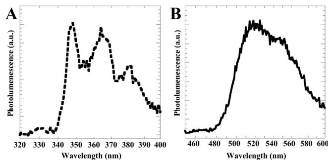
Figure 4. Photoluminescence spectra of magnetic nanoparticles modified with two dyes simultaneously. A) The excitation of carbazole was observed at 348 and 363 nm and B) the excitation of the fluorescein dye was observed at 517 nm.
