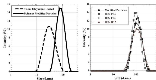
Figure 2. (Left) Hydrodynamic diameter by intensity of magnetic nanoparticles before and after modification with Alkyne-PEO-NitroDOPA(6); size data chart available (Table S1). (Right) Hydrodynamic diameter by intensity of the particles titrated with PBS, FBS, and BSA.
