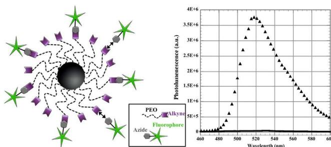
Figure 3. Image on the left represents the final construction of magnetic nanoparticle with functional surface modified with a fluorophore. Image on the right shows a photoluminescence spectrum of particles before and after functionalization with fluorescein.
