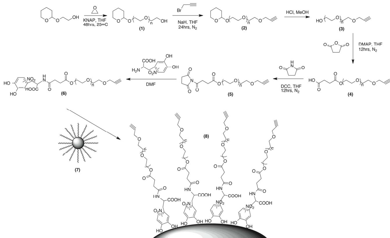
Figure 1. Synthesis of Heterobifunctional PEO with alkyne on one end and NitroDOPA on the other
