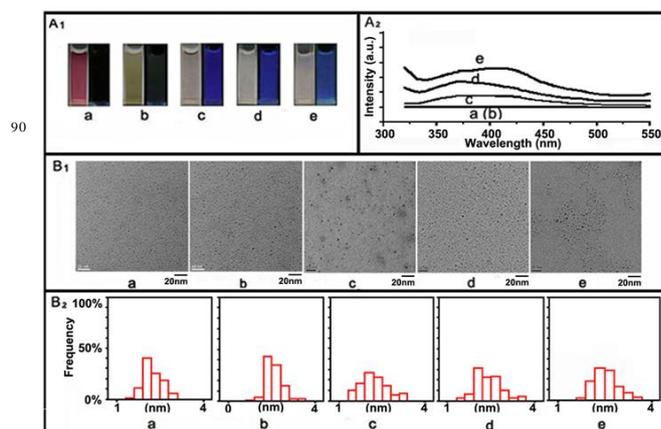
Figure 1. Characterisation of the five colloidal metal NPs (a: Au NPs; b: Ag NPs; c: Cu NPs; d: Ni NPs and e: Co NPs) (A<sub>1</sub>) Photographs taken under the sunlight and ultraviolet light at  $312 \pm 10 \text{ nm}$  excitation, respectively; (A<sub>2</sub>) Fluorescence emission spectra excited at  $312 \text{ nm}$ ; (B<sub>1</sub>) Typical TEM images and (B<sub>2</sub>) particle size distributions.
