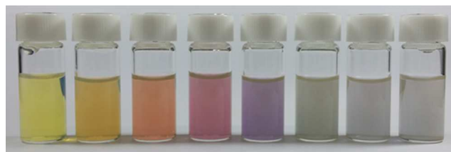
Fig. 6. Photographs of aqueous dispersions of Ag nanoplates grown in the presence of iodide ions. The times, during the nanoplate growth process, at which the iodide solutions were added to the reaction solution were (from left to right): t = 0 h, t = 1 h, t = 1.3 h, t = 1.6 h, t = 2 h, t = 3 h, or t = 4 h after the reaction had begun. The sample farthest to the right was prepared without adding iodide ions.
