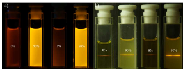
Fig. 11 a) The one-photon fluorescence (OPF) emission photos of TABzPA and TATpPA at a concentration of 1 \times 10^{-5} M, respectively, in different ratio of water in THF under 365 nm light illumination. b) The two-photon emission (TPF) emission images of TABzPA and TATpPA , respectively, in the different ratio of water in THF excited at 800 nm laser.
