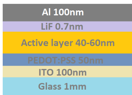
Figure 4 PLED device stack, ITO: Indium-Tin Oxide.
