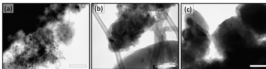
**Figure 2** TEM images of carbon structure on nickel mesoporous layer after (a) 400°C, (b) 600°C, and (c) 800°C growth. The scale bars show 50 nm.
