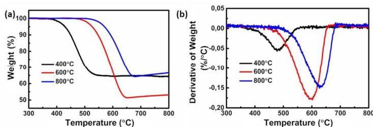
**Figure 4** (a) Weight and (b) differential thermal gravimetric curves for different nanostructured Ni-carbon composites.
