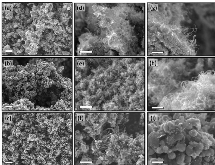
**Figure 1** SEM images of porous structure of carbon growth on nickel mesoporous layer at (a, d, g) 400°C, (b, e, h) 600°C, (c, f, i) 800°C, the scale bar of (a-c), (d-f) and (g-i) are 10  $\mu\text{m}$ , 1  $\mu\text{m}$  and 400 nm, respectively.
