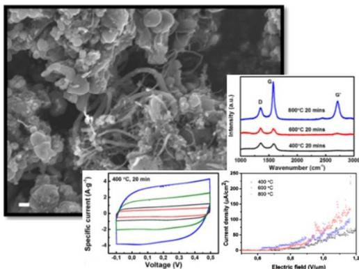
Films of porous Raney nickel catalyst particles deposited on various substrates by stencil printing from dispersions of the catalyst and poly(methyl methacrylate) in 2-(2-butoxyethoxy)ethyl acetate offer a facile platform for synthesizing nanostructured carbon-nickel composites for direct use as electrodes in electrochemical applications as well as in field emitter devices.
