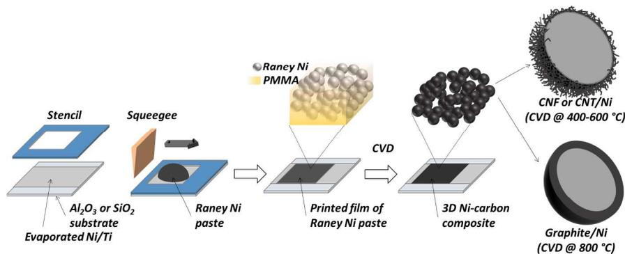
**Scheme 1** Schematic drawing of the fabrication process including evaporation of under-metallization, stencil printing the catalyst and subsequent chemical vapor deposition of nanostructured carbons.
