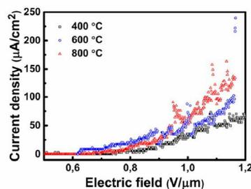
**Figure 6** Field emission of carbon/Raney nickel composites.
