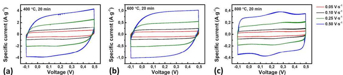
**Figure 5** Cyclic voltammetry curves with different charge/discharge rates of carbon grown on nickel mesoporous layer after (a)  $400^\circ\text{C}$ , (b)  $600^\circ\text{C}$ , and (c)  $800^\circ\text{C}$  growth process.
