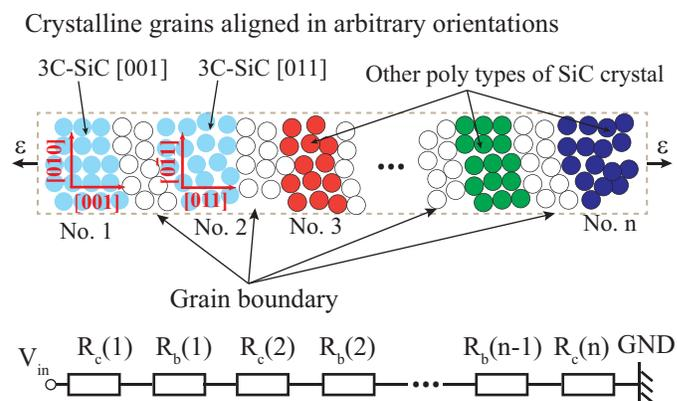
**Fig. 4** An one dimensional (1-D) model of the crystalline structure of nc-SiC which contains a large number of crystalline SiC grains and grain-boundary.
