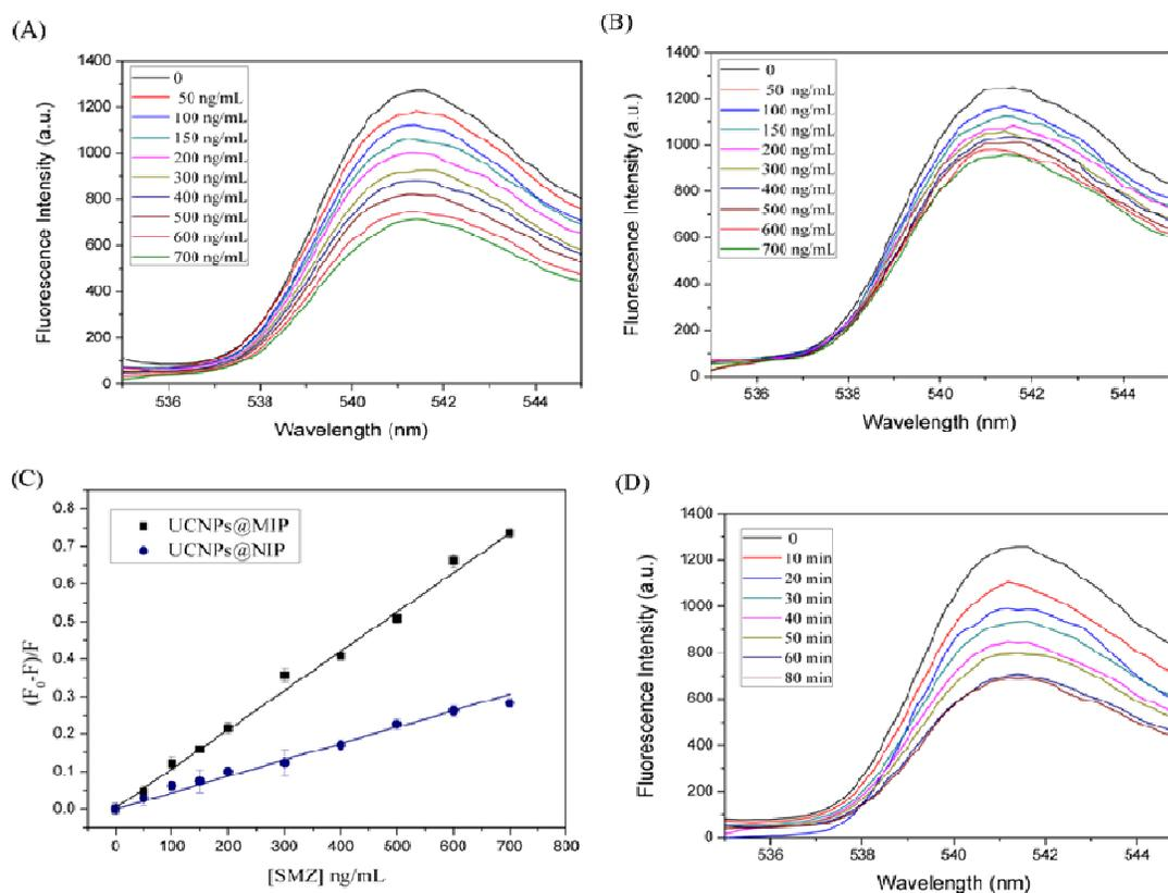
Fig 5. Fluorescence spectra of UCNPs@MIP (A) and UCNPs@NIP (B) at various SMZ concentrations. (C) Stern–Volmer plot of UCNPs@MIP and UCNPs@NIP. (D) Fluorescence spectra of the UCNPs@MIP in the presence of SMZ ( $1 \mu\text{g mL}^{-1}$ ) after incubating for different times.
