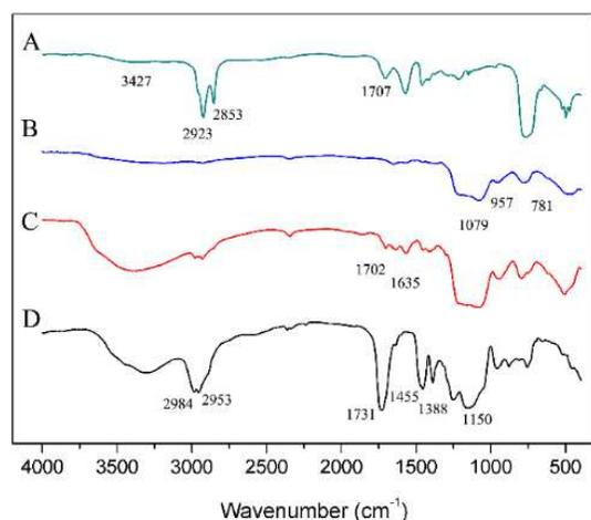
Fig 3. FT-IR spectra of OA-UCNPs (A), UCNPs@SiO<sub>2</sub> (B), vinyl modified-UCNPs@SiO<sub>2</sub> (C) and UCNPs@MIP (D).
