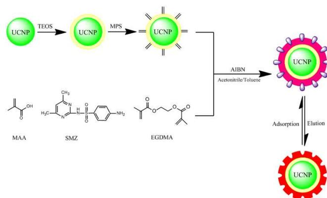
Fig 1. Schematic illustration of the synthetic procedure of UCNPs@MIP
