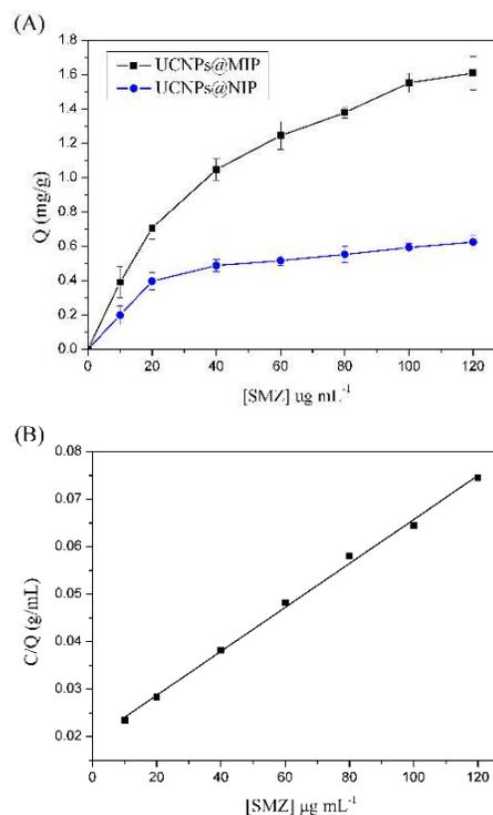
Fig 4. Adsorption isotherms of the UCNPs@MIP and UCNPs@NIP at 25°C (A); Langmuir plot of UCNPs@MIP towards SMZ (B).
