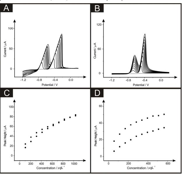
Linear sweep voltammograms resulting from additions of lead (II) (103.61 to 932.42  $\mu g L^{-1}$ ) and cadmium (II) (56.46 to 508.14  $\mu g L^{-1}$ ) into a pH 4.3 acetate buffer solution (dotted line) containing 5 mg $L^{-1}$  of antimony (III) using both an SPE (A) and BDDE (B). Also depicted are the corresponding calibration plots for lead (II) (C) and cadmium (II) (D) at the SPE (squares) and BDDE (circles). Deposition potential and time: - 1.2 V (vs. SCE) and 120 seconds respectively.
