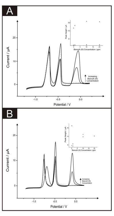
Linear sweep voltammograms resulting from additions of lead (II) (103.61 to 932.42  $\mu g L^{-1}$ ) and cadmium (II) (56.46 to 508.14  $\mu g L^{-1}$ ) into a pH 4.3 acetate buffer solution (dotted line) using both a bare SPE (A) and a bare BDDE (B). Also depicted are the corresponding calibration plots for lead (II) (C) and cadmium (II) (D) at the SPE (squares) and BDDE (circles). Deposition potential and time: - 1.2 V (vs. SCE) and 120 seconds respectively.
