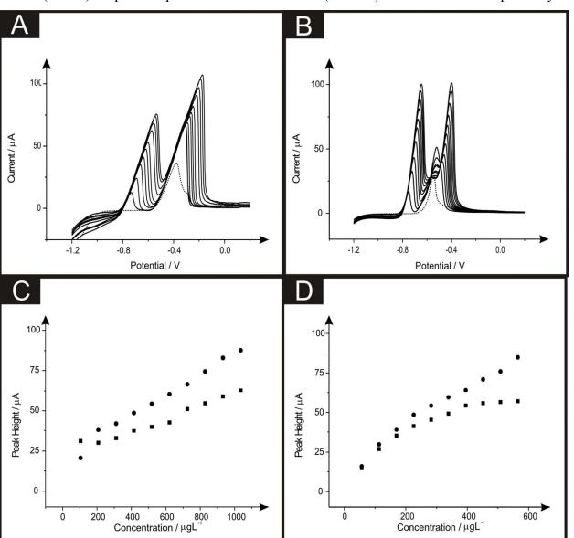
Linear sweep voltammograms resulting from additions of lead (II) (103.61 to 932.42  $\mu g L^{-1}$ ) and cadmium (II) (56.46 to 508.14  $\mu g L^{-1}$ ) in to a pH 4.3 acetate buffer solution (dotted line) containing 1 mg $L^{-1}$  of bismuth (III) using both an SPE (A) and BDDE (B). Also depicted are the corresponding calibration plots for lead (II) (C) and cadmium (II) (D) at the SPE (squares) and BDDE (circles). Deposition potential and time: - 1.2 V (*vs.* SCE) and 120 seconds respectively.
