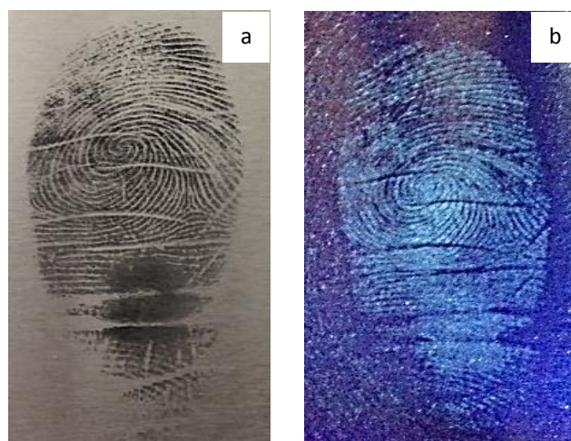
Fig. 1 Images of Anadin Extra spiked fingermarks from the same donor dusted using a magnetic applicator with (a) Black magnetic powder photographed under normal light and with (b) CHCA magnetic powder photographed under UV light, 254 nm
