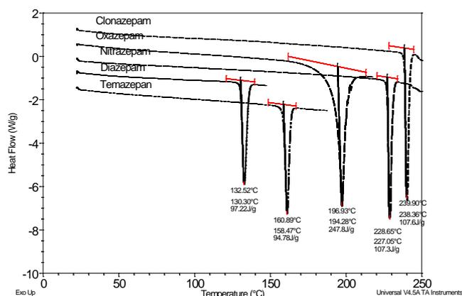
Fig.3 DSC thermograms of five different benzodiazepines at a heating rate of 10°C/min indicating the individual melting points. Values of  $T_{onset}$  and  $T_{max}$  and the enthalpy of fusion (J/g) are indicated for each pure compound.
