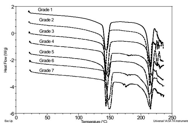
Fig.5 Grade1– Lactose B.P. (supplier unknown); Grade 2 Granulac™230; Grade 3 - Lactopress™150; Grade 4 - Lactopress™SD; Grade 5-Pharmatose™80; Grade 6 - Lactopress™175; Grade 7-Lactopress™300.
