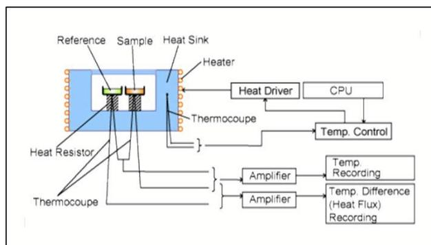
Fig. 1 Schematic diagram of a heat flux differential scanning calorimeter (DSC). Courtesy of Hitachi-Hightec.com
