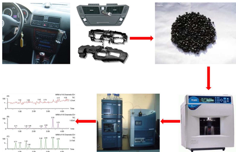
A UPLC-MS/MS method combined with MAE for detection of OPEs in automobile Interiors. The method is rapid, effective and eco-friendly. 39x25mm (600 x 600 DPI)
