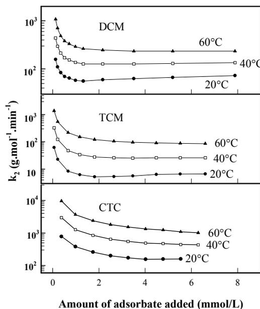
**Fig. 10** Dependence of the adsorption rate constants of the pseudo-second-order model on the amounts of adsorbate added and temperature.
