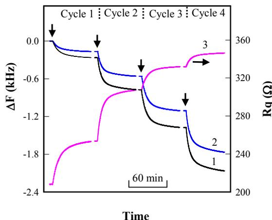
**Fig. 3** Changes in frequency and motional resistance of QCM during the processes of growth ZIF-8 films. The arrow indicates the start of a new fabrication cycle by addition of fresh mixture of 25 mM  $Zn^{2+}$  and 50 mM mIM in the cell. (1): measured frequency shift (black); (2): corrected frequency shift (blue); (3): motional resistance (pink).
