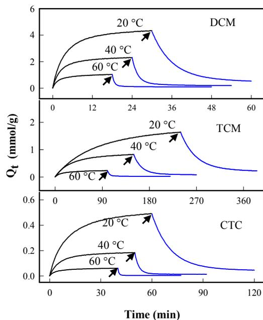
**Fig. 6** Influence of temperature on the amount adsorbed in ZIF-8 film ( $0.70\mu\text{m}$ ) in adsorption and desorption processes. The inclined arrows indicate the start of an exhaustion process using vacuum pump. The amounts of DCM, TCM and CTC added were 0.716, 1.17 and 1.74  $\text{mmol}/\text{L}$ , respectively.
