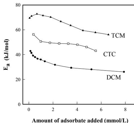
**Fig. 11** Dependence of the adsorption activation energy on the amounts of adsorbate added.
