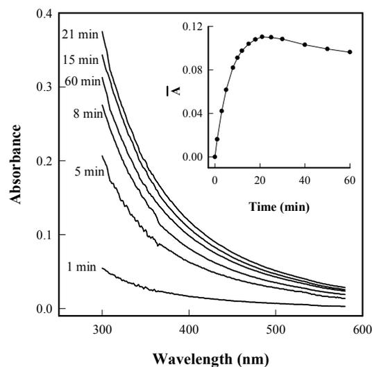
**Fig. 4** Changes in absorbance spectrum of the reaction mixture during the processes of growth ZIF-8 films. Inset: Change of the averaged absorbance with the reaction time.
