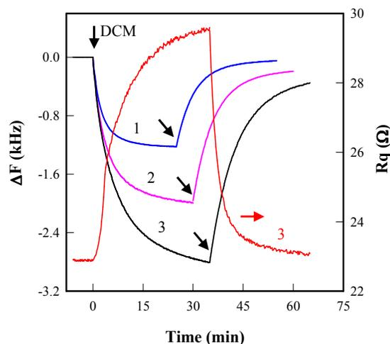
**Fig. 5** Changes of the frequency and motional resistance of QCM in the processes of the adsorption and desorption of TCM on ZIF-8 film ( $20^\circ\text{C}$ ). ZIF-8 film thickness: (1):  $h=0.36 \mu\text{m}$ ; (2):  $h=0.70 \mu\text{m}$ ; (3):  $h=1.28 \mu\text{m}$ . The amount of DCM was  $0.716 \text{ mmol}/\text{L}$ . The inclined arrows indicate the start of an exhaustion process using vacuum pump.
