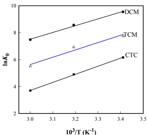
**Fig.12** Determination of adsorption enthalpy of DCM, TCM and CTC on ZIF-8 film (0.70 $\mu$ m).
