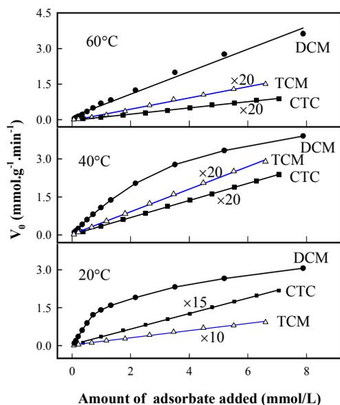
**Fig. 9** Dependence of the initial rate of adsorption on the amounts of adsorbate added and temperature.
