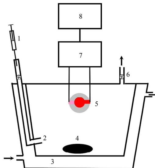
**Fig. 2** Schematic drawing of experimental setup employed for the adsorption measurements (not to scale). (1): syringe with organic solvent; (2): inlet for adsorbate vapor; (3): thermostatic water bath; (4): magnetic mixer; (5): QCM sensor with ZIF-8 film; (6): vacuum pump; (7): impedance analyzer; (8): computer.
