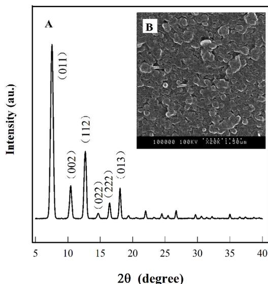
**Fig. 1** Powder XRD patterns of as-prepared ZIF-8 crystal (A) and scanning electron micrographs of the surface of the as-synthesized ZIF-8 film (B).
