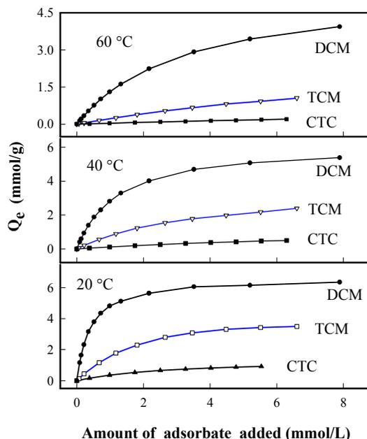
**Fig.8** Adsorption isotherms of DCM, CTM and CTC in ZIF-8 film (0.70 $\mu$ m) at different temperature.
