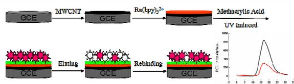
**Scheme 1.** The fabrication process of the MIP-ECL sensor and the detecting of OTA.
