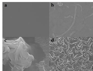
**Figure 1.** SEM images of the modified electrode. (a) The bare electrode, (b) MWCNTs/Nafion/GCE, (c)  $\text{Ru}(\text{bpy})_3^{2+}$ /MWCNTs/Nafion/GCE, (d) MIP/ $\text{Ru}(\text{bpy})_3^{2+}$ /MWCNTs/Nafion/GCE.
