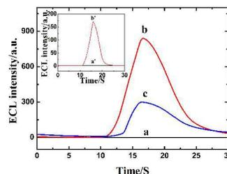
**Figure 3.** ECL curves of (a) MIP/Ru(bpy)<sub>3</sub><sup>2+</sup>/MWCNTs/Nafion/GCE before template removal, (b) MIP/Ru(bpy)<sub>3</sub><sup>2+</sup>/MWCNTs/Nafion/GCE after template removal, (c) MIP/Ru(bpy)<sub>3</sub><sup>2+</sup>/MWCNTs/Nafion/GCE after rebinding. Inset: the ECL curves of (a') NIP/Ru(bpy)<sub>3</sub><sup>2+</sup>/MWCNTs/Nafion/GCE, (b') NIP/Ru(bpy)<sub>3</sub><sup>2+</sup>/MWCNTs/Nafion/GCE after template removal.
