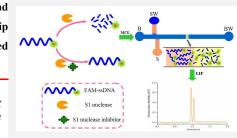
A novel microchip electrophoresis method with laser induced fluorescence detection was developed for ultrasensitive detection of nuclease activity and inhibitor.
