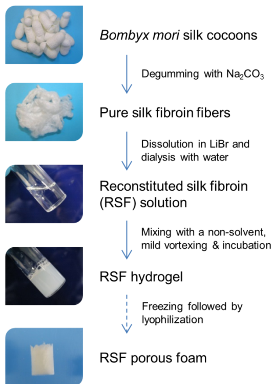
Figure 1. Schematic of the NIPS induced RSF hydrogels and porous foams preparation: B. mori cocoons were first degummed in the boiling sodium carbonate solution to yield the pure fibroin fibers. The fibers were dissolved in the lithium bromide solution and the mixture was dialyzed against water to yield the aqueous solution of reconstituted silk fibroin or RSF. RSF solution was mixed with a definite amount of methanol and subjected to mild vortexing and then incubated at a preset temperature to become hydrogels. The hydrogels were collected and rinsed with water to washout the traces of methanol. Alternatively, the hydrogels may be subjected to freeze-drying to yield the porous foams.
