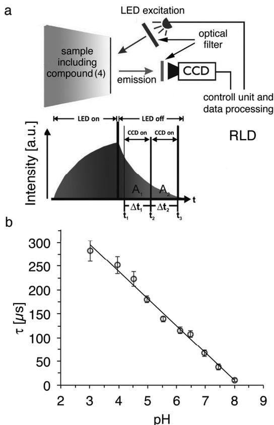
**Figure 3.** (a) Scheme of the instrumental set up and measurement principle (RLD) of the time-gated luminescence imaging method applied for the determination of the luminescence lifetime changes of (4) to pH. For details
