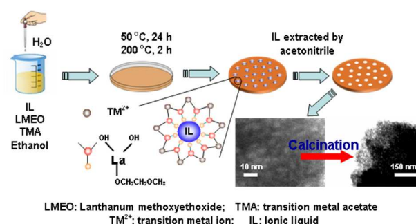
Scheme. 1 The synthesis process for mesoporous lanthanum transition metal perovskite oxides by an ionic liquid
