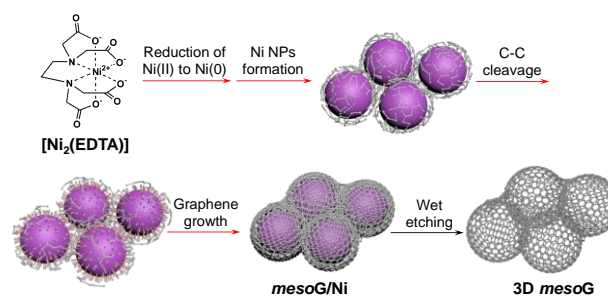
Scheme 1. Schematic representation of the thermal conversion of [Ni 2 (EDTA)] into three-dimensional mesoporous graphene, 3D mesoG . The processes indicated by red arrows occurred during the one-step heat treatment of [Ni 2 (EDTA)].
