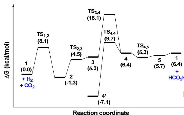
**Fig. 3** Free energy profile for the formation of formic acid from H<sub>2</sub> and CO<sub>2</sub> catalyzed by **1**.
