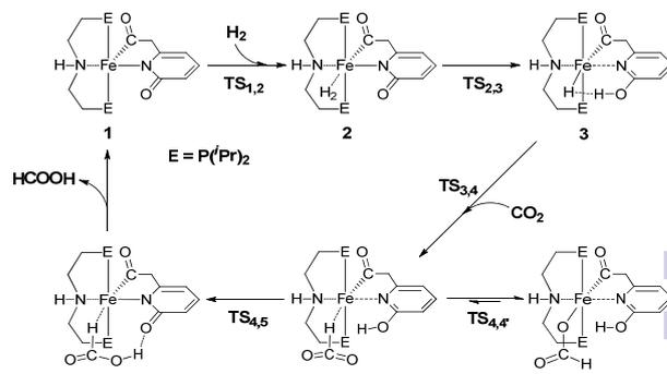
**Scheme 1** Mechanism of hydrogenation of CO<sub>2</sub> catalyzed by newly designed pincer iron complexes features the formation of a strong Fe-H<sup>δ-</sup>...H<sup>δ+</sup>-O dihydrogen bond for H<sub>2</sub> cleavage.
