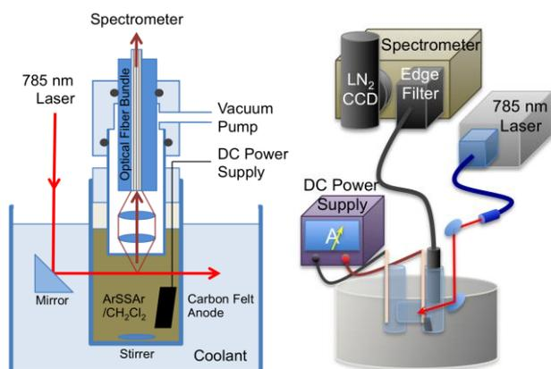
**Fig. 1** Schematics for the optical probe operated at 195 K (left) for the *in situ* Raman spectroscopic measurement system (right).
