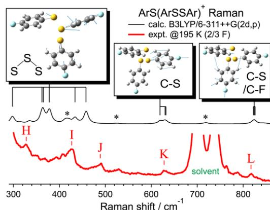
**Fig. 5** The experimental spectrum (thick line in red) at 2/3 F of electricity showing bands H-L for ArS(ArSSAr)<sup>+</sup> (Ar = *p*-FC<sub>6</sub>H<sub>4</sub>) compared with the calculated Raman spectrum at B3LYP/6-311++G(2d,p) (thin line in black).<sup>13</sup> Displacement vectors are illustrated for three normal modes of S-S, C-S, and C-S/C-F vibrations. Asterisks indicate weak Raman modes of out-of-plane ring deformations. Calculated vibrational frequency is scaled by a factor of 0.98.
