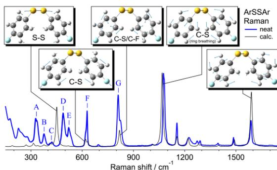
**Fig. 2** Raman spectrum of ArSSAr (Ar =  $p\text{-FC}_6\text{H}_4$ ) (neat) at ambient temperature before electrolysis (thick line in blue) compared with the calculated Raman spectrum at B3LYP/6-311++G(2d,p) level of theory<sup>13</sup> (thin line in black). The calculated frequency is scaled by a factor of 0.98 for possible anharmonicity. Insets show calculated displacement vectors for each of the selected normal mode vibrations.
