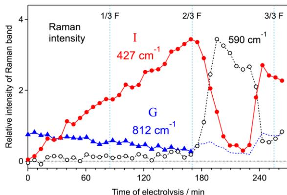
**Fig. 4** Intensity profiles of selected Raman bands as a function of time of electrolysis. Current for the electrolysis was fixed at 8.0 mA throughout the experiment. Plots correspond to the band I for sulfonium ion, ArS(ArSSAr)<sup>+</sup>, (●), the band G for disulfide, ArSSAr, (▲), and the band at 590 cm<sup>-1</sup> for a by-product (○).
