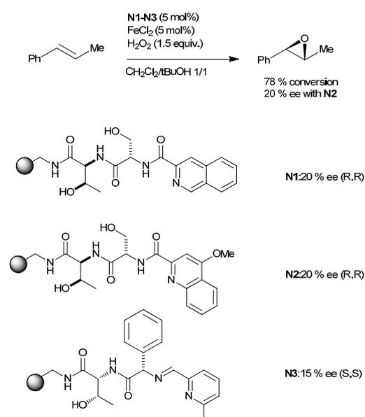
**Scheme 1.** Asymmetric epoxidation of *trans*- $\beta$ -methylstyrene with peptide **N1-N3** ligands using  $\text{H}_2\text{O}_2$  as oxidant.<sup>37</sup>
