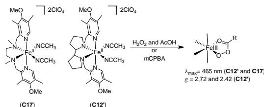
**Scheme 8.** Synthesis of acylperoxoiron(III) complexes from reaction of  $[Fe^{(DMM)men}(CH_3CN)_2](ClO_4)_2$  (**C17**) and  $[Fe^{(DMM)PDP}(CH_3CN)_2](ClO_4)_2$  (**C12'**) with H<sub>2</sub>O<sub>2</sub>/AcOH or peracids.
