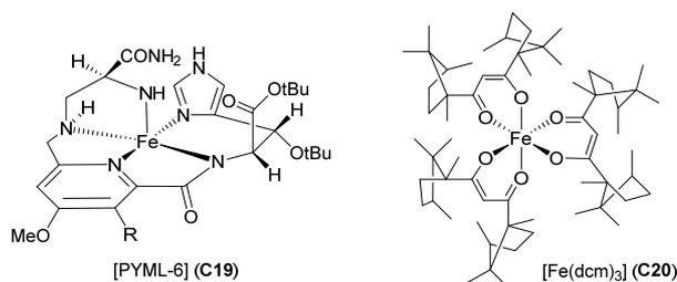
Figure 5. Iron catalysts that employ O<sub>2</sub> to perform asymmetric epoxidation.
