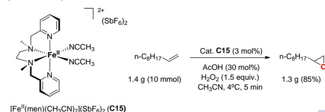
**Scheme 5.** Epoxidation of aliphatic alkenes using **C15** with hydrogen peroxide and acetic acid on gram scale
