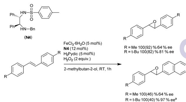
**Scheme 2.** Asymmetric epoxidation of *trans*-stilbene derivatives using diamine **N4**,  $\text{FeCl}_3 \cdot 6\text{H}_2\text{O}$ ,  $\text{H}_2\text{O}_2$  and dipicolinic acid.<sup>39,4</sup> 4 equiv.  $\text{H}_2\text{O}_2$ , 10 mol %  $\text{H}_2\text{pydic}$ , 5 mol %  $\text{FeCl}_3 \cdot 6\text{H}_2\text{O}$ , 24 mol % **N4**. Reaction at  $10^\circ\text{C}$
