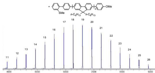
**Figure 1a.** Maldi-tof spectrum of polyfluorene with *p*-MeOC<sub>6</sub>H<sub>4</sub>/*o*-MeSC<sub>6</sub>H<sub>4</sub>C<sub>6</sub>H<sub>4</sub> as two end groups.
