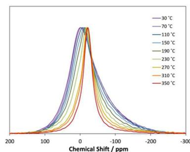
Figure 1: <sup>23</sup>Na solid state NMR spectra recorded at temperatures from 30 to 350 °C in 40 °C increments for a sample of nominal composition Sr<sub>0.6</sub>Na<sub>0.4</sub>SiO<sub>2.8</sub>. Peak heights have been normalised.
