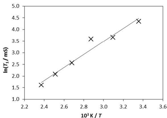
Figure 2: Arrhenius plot of  $T_1$  relaxation times of  $^{23}\text{Na}$  recorded at temperatures from 25 to 150 °C in 25 °C increments for a sample of nominal composition  $\text{Sr}_{0.6}\text{Na}_{0.4}\text{SiO}_{2.8}$ . The one-standard deviation uncertainties associated with random noise are of the order of the size of the symbols used.
