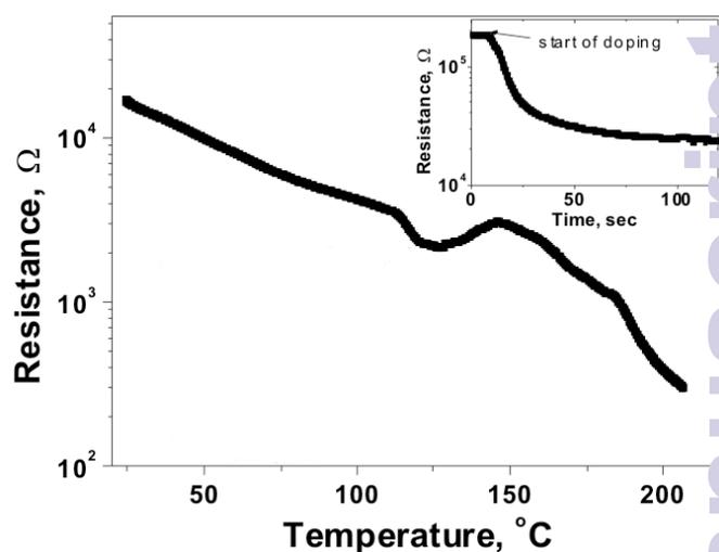
Fig. 3 (a) Temperature dependence of the resistance for a doped  $\text{CuCl}_2$  xerogel of **1** during the annealing (main panel). Top inset shows typical dependence of resistance vs time during doping by iodine vapor at room temperature.
