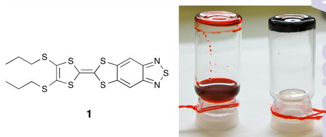
**Fig. 1** (Left) chemical structure of the gelator **1**; (Right) photograph showing, in the left vial, the control experiment of **1** in chloroform and ethanol with no metal salt added and in the right vial, upon addition of CuCl<sub>2</sub>.
