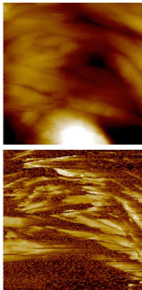
Fig. 4 Topography (top) and current (bottom, bias voltage 1.1 V) images from CS-AFM of the same region ( $3 \times 3$  microns) of a  $\text{CuCl}_2$  xerogel of **1** on highly oriented pyrolytic graphite. The brighter regions in the current map correspond to high conductivity. The independence of the responses is highlighted by the insulating bump in the topographic image.
